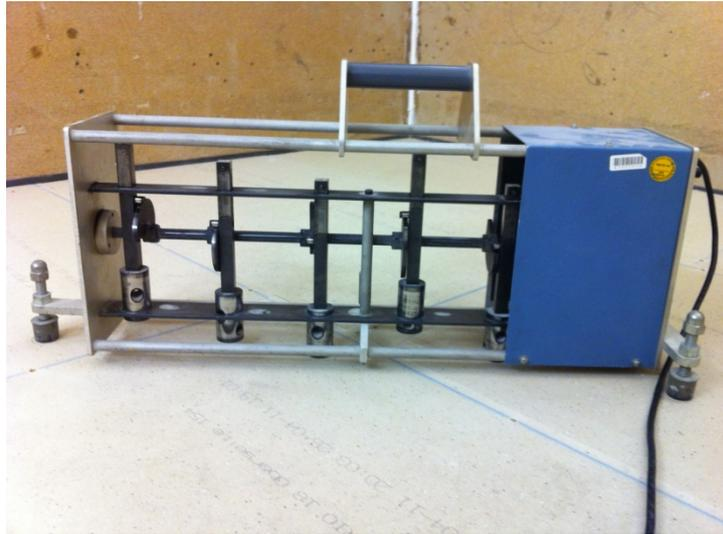
Figure 1: Photograph of the utilised tapping machine.
