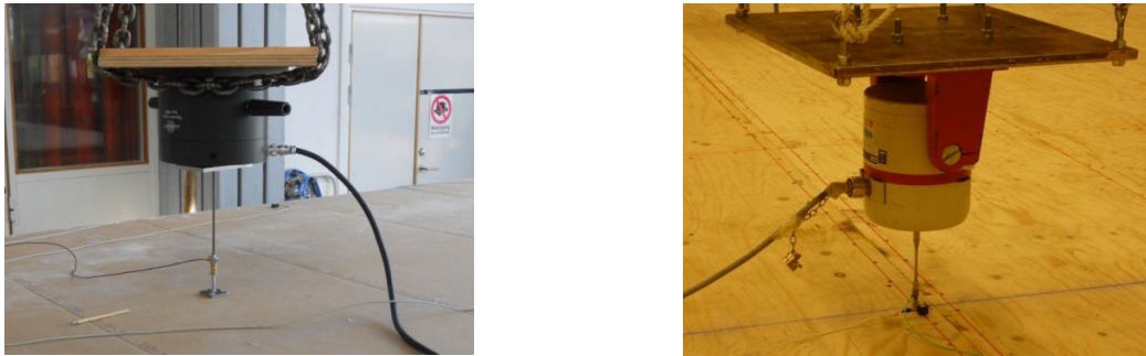
Figure 10. Shakers used to excite the floors to the left dynamic tests performed in Lund and to the right in Växjö.
