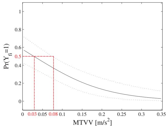
Figure 27: Vibration acceptability model involving MTVV – Overall regression line. —: median value; - - : lower and upper limits of the 95% credibility interval.
