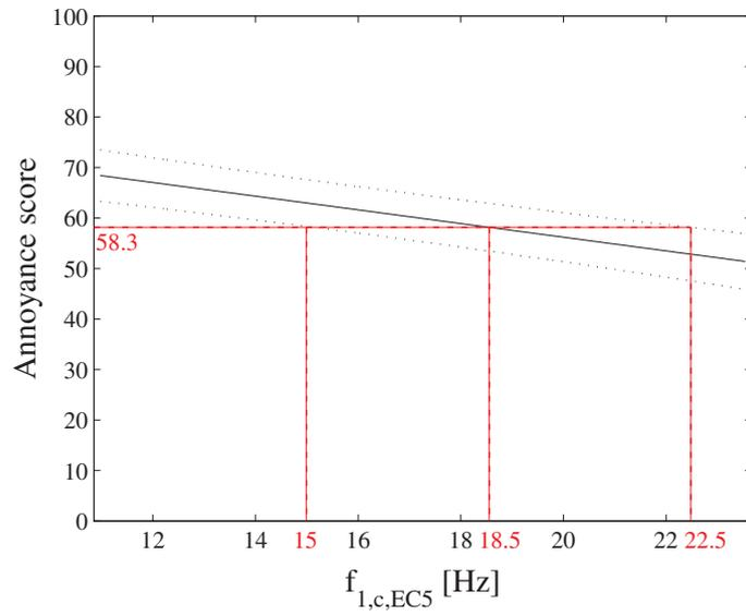
Figure 25: Vibration annoyance model involving  $f_{1,c,EC5}$  – Overall regression line. —: median value; - - : lower and upper limits of the 95% credibility interval.
