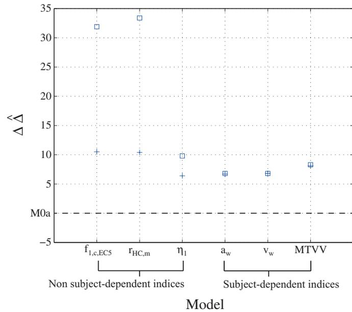
Figure 21: Vibration acceptability - Differences in  $\hat{\Delta}$  ( $\Delta \hat{\Delta}$ ) between null model  $M0$ , and the models involving occasion-level predictors. +: fixed-slope model; □: random-slope model.
