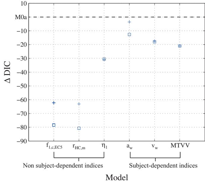
Figure 18: Vibration annoyance - Differences in DIC ( $\Delta$ DIC) between null model  $M0$ , and the models involving occasion-level predictors. +: fixed-slope model; □: random-slope model.
