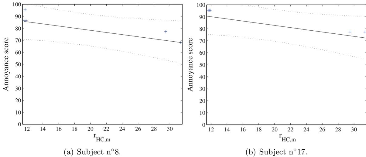
Figure 23: Vibration annoyance model involving  $r_{HC,m}$  – Individual regression lines for two subjects. —: median value; - -: lower and upper limits of the 95% credibility interval;+: actual scores.
