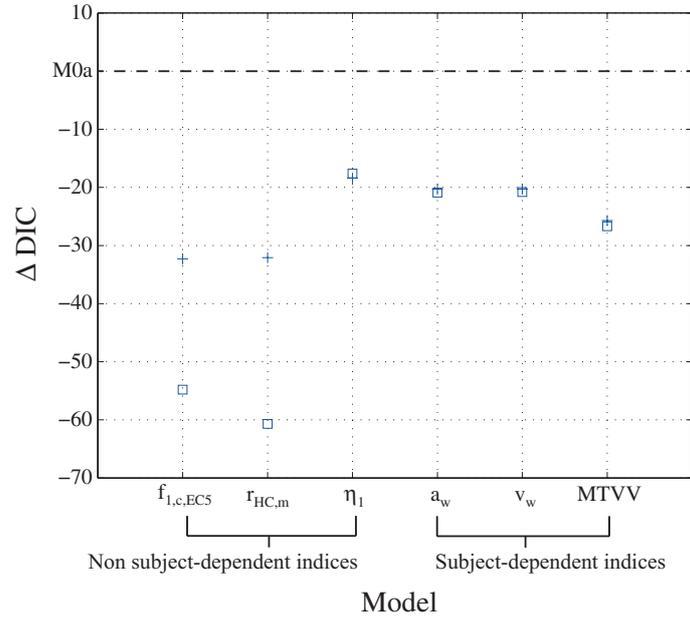
Figure 20: Vibration acceptability - Differences in DIC ( $\Delta DIC$ ) between null model  $M0$ , and the models involving occasion-level predictors. +: fixed-slope model; □: random-slope model.
