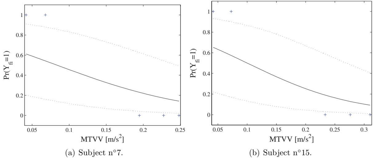
Figure 24: Vibration acceptability model involving MTVV – Individual regression lines for two subjects. —: median value; - - : lower and upper limits of the 95% credibility interval; +: actual binary responses.
