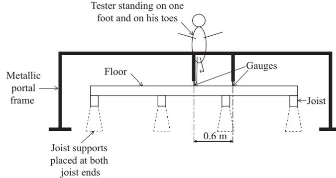
Figure 12: Side view of the floortop deflection measurement setup.
