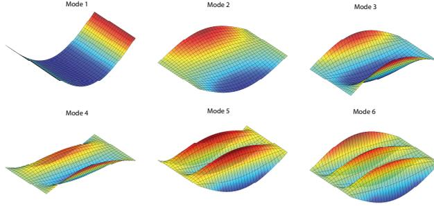
Figure 15: Eigenmodes for Floor E calculated with Calvem.
