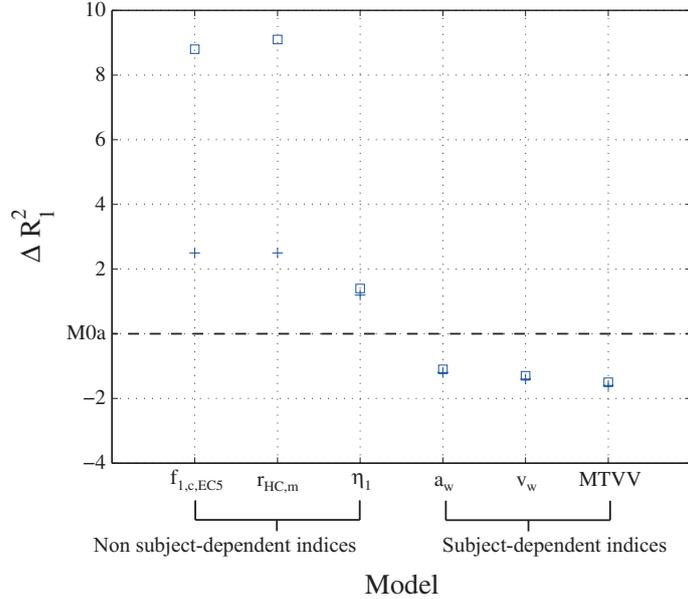
Figure 19: Vibration annoyance - Differences in  $R_1^2$  ( $\Delta R_1^2$ ) between null model  $M0$ , and the models involving occasion-level predictors. +: fixed-slope model; □: random-slope model.
