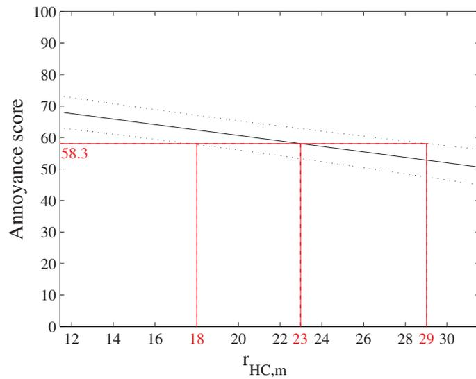
Figure 26: Vibration annoyance model involving  $r_{HC,m}$  – Overall regression line. —: median value; - - : lower and upper limits of the 95% credibility interval.
