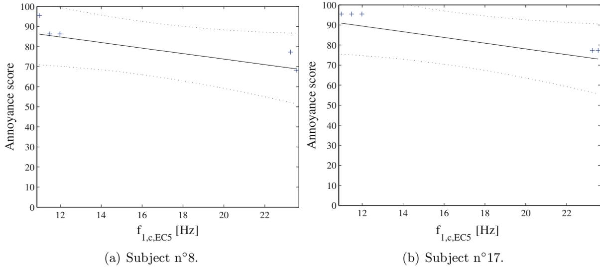
Figure 22: Vibration annoyance model involving  $f_{1,c,EC5}$  – Individual regression lines for two subjects. —: median value; - -: lower and upper limits of the 95% credibility interval;+: actual scores.
