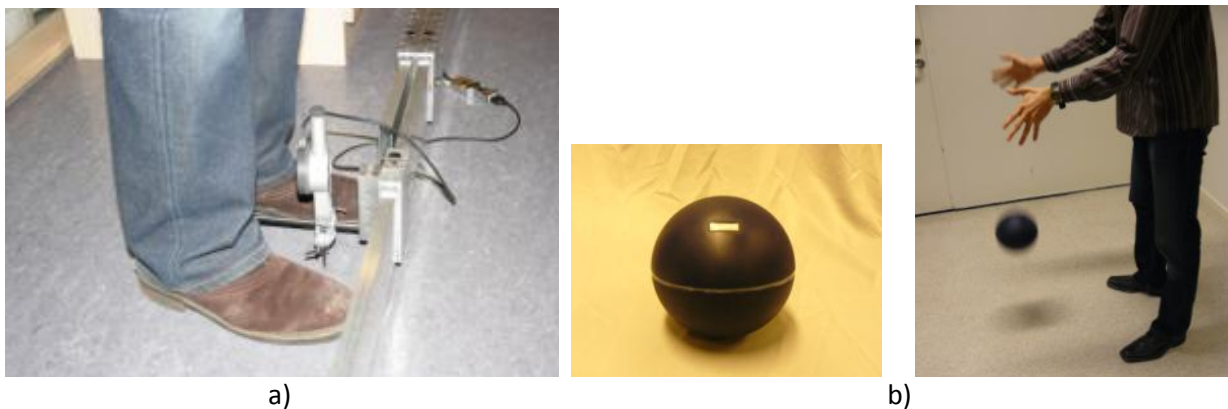
Figure 6. a) Measurement of floor deflection due to a point load and b) vibration excitation with standardized impulse ball.
