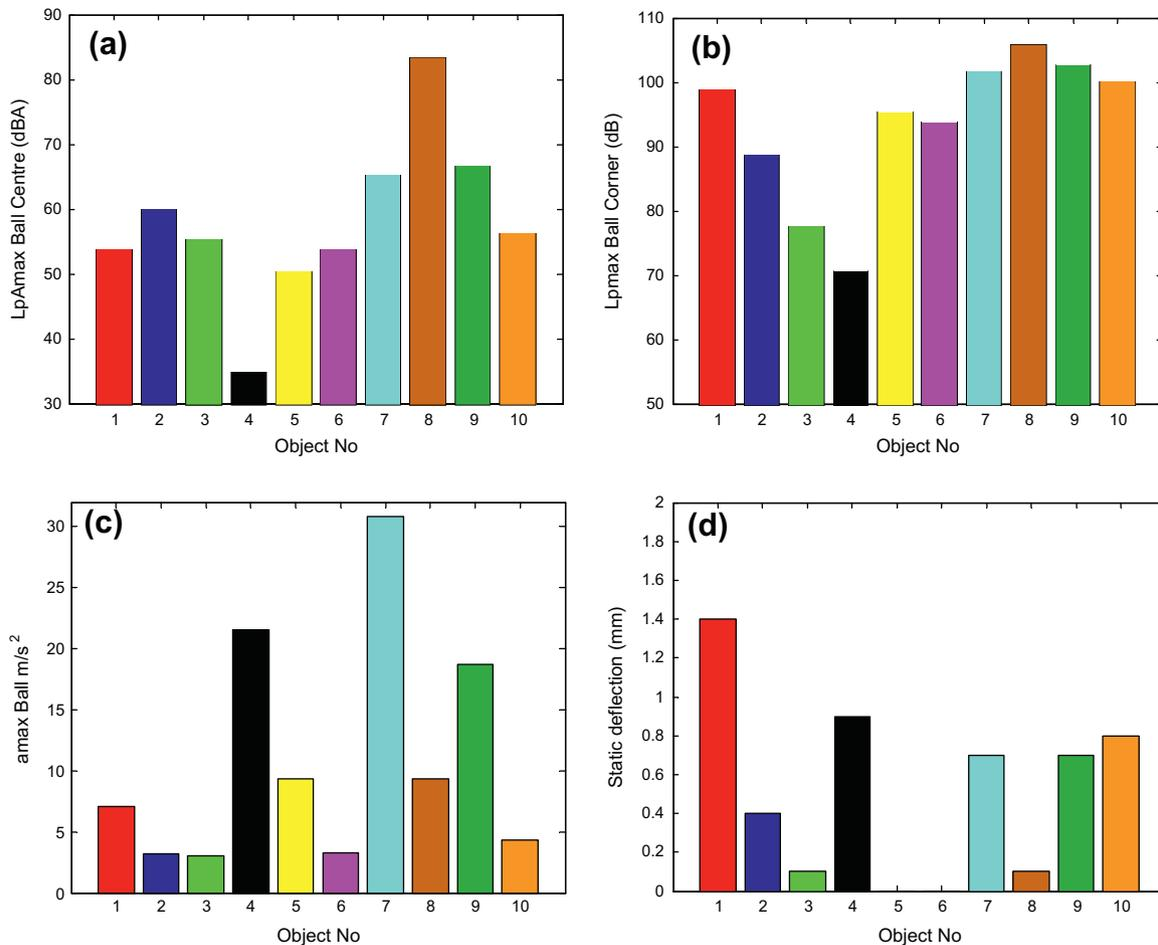
**Fig. 3.** Alternative measurements; (a) rubber ball, A-weighted sound in the centre of the receiving room (b) rubber ball, sound in one corner of the receiving room, (c) rubber ball, floor vibrations and (d) Static deflection due to a 1 kN load.
