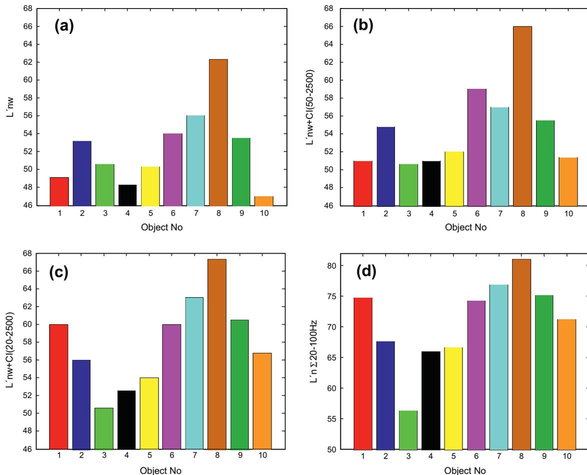
**Fig. 2.** Impact sound insulation; (a)  $L'_{n,w}$ , (b)  $L'_{n,w} + C_{I,50-3150}$ , (c)  $L'_{n,w} + C_{I,20-2500}$  and (d)  $L'_{n, \sum_{20-100}}$  ( $L'_{n,w}$  is evaluated according to the Swedish national standard.).
