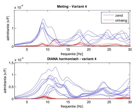
Figure 4: Comparison between the measured and the predicted transfer mobility of the junction with floor screed. (see figure 3 for the meaning of words)
