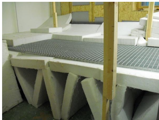
Figure 1: sound absorption layer opposite the measurement surface
