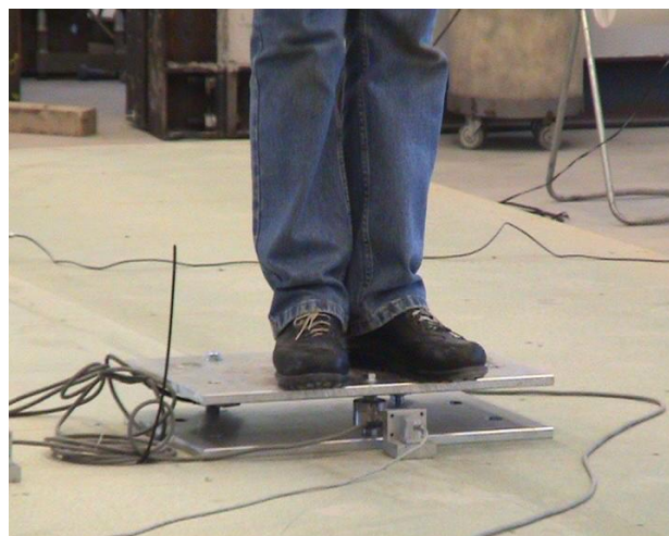
Figure 5: Plateau with force cells to measure the force during a heeldrop-test.
