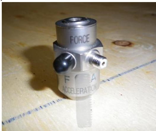
Figure 5.3: Accelerometer mounted using a double sided threaded stud
