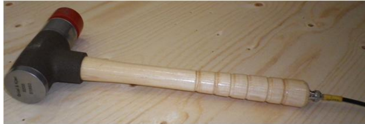
Figure 5.1: The modal hammer used for all experimental studies
