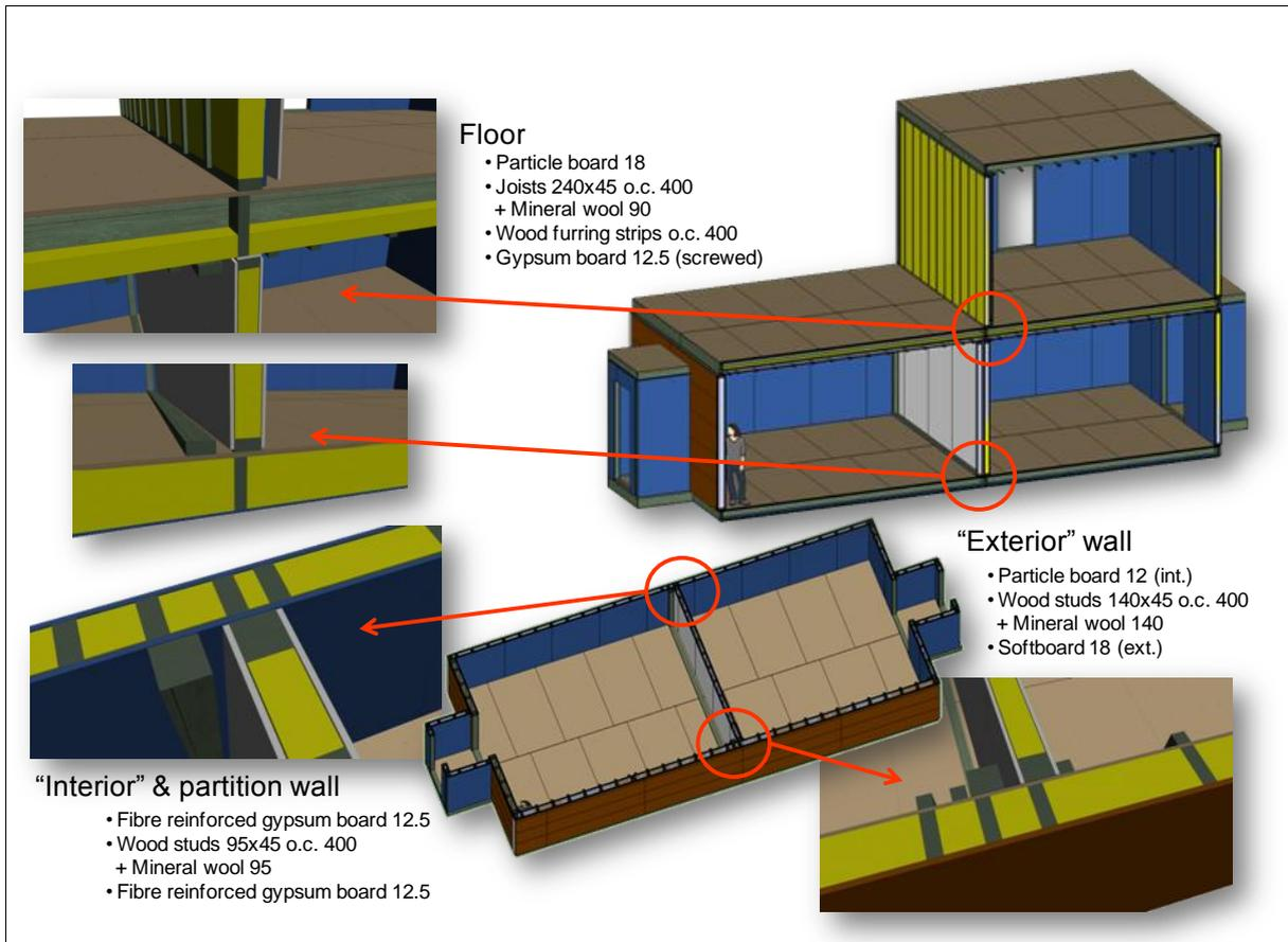
Figure 45 a: Timber frame mock-up at Machiels Building Solutions at Beringen (Belgium) (all dimensions in mm)
