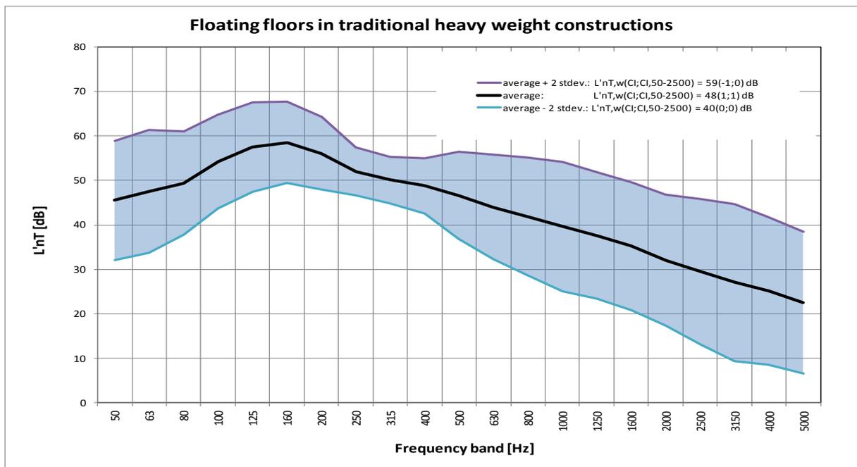
Graph 4: Average spectrum of the standardised impact sound pressure level  $L'_{nT}$  measured in situ on 20 well-executed traditional floating floors in Belgium. 95% of the measured values are situated inside the shaded zone.
