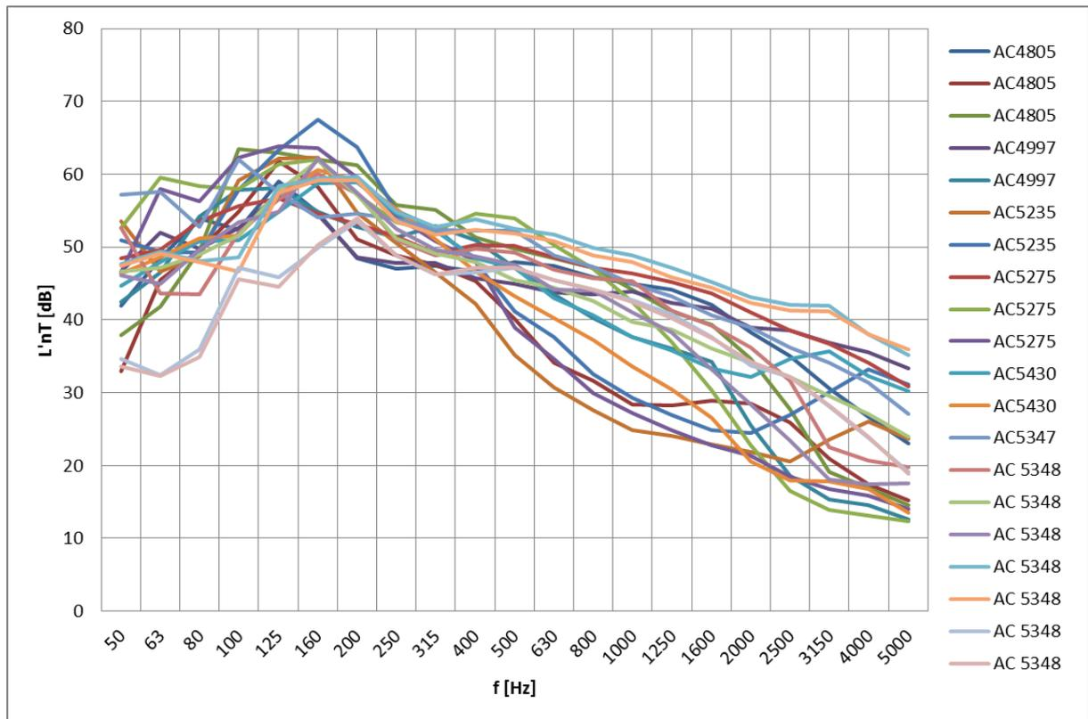
Graph 2: Average spectrum of the standardised impact sound pressure level  $L'_{nT}$  measured in situ on 20 well-executed traditional floating floors in Belgium.
