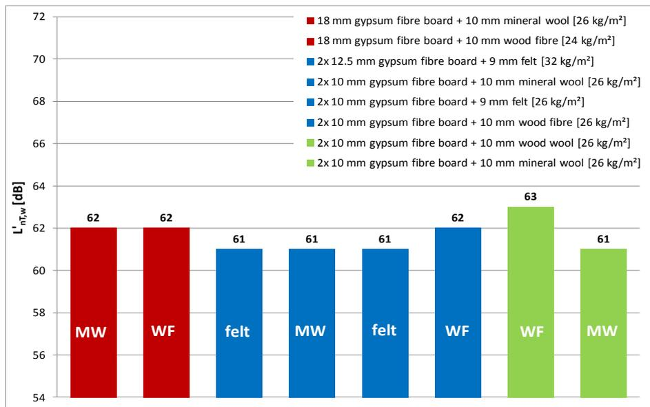
Chart 9: single value results for different pre-assembled dry floating floor systems tested on reference floor
