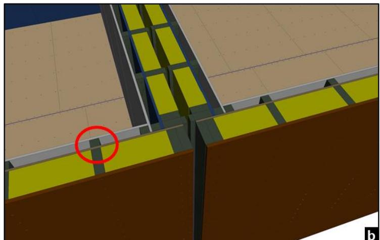
Figure 24: technical lining can be beneficial (picture b) but can present dangers such as the heavy technical lining for bathrooms with thick, very rigid steel studs, to which vibration sources (sinks, toilet...) will be attached (picture a).
