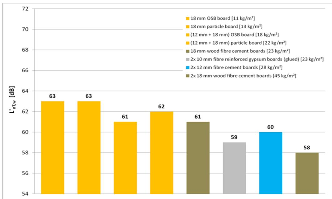
Chart 1: different board types tested on top of a 20 mm thick mineral wool layer (140 kg/m<sup>3</sup>)
