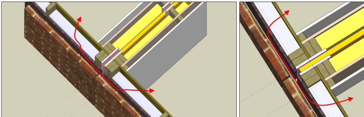
Figure 28: transmission path 1 for the indirect sound transmission, this transmission path is important when thermal insulation is used with no acoustic absorbent characteristics.
