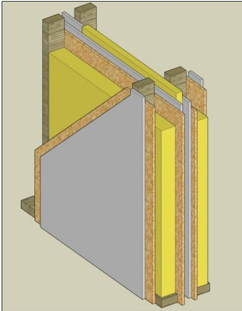
Composition: central cavity of 20 mm cavity filled with mineral wool 20 mm ca.  $16 \text{ kg/m}^3$  with symmetrically on both sides of the cavity (going from the inside towards the outside): 1x12.5 mm fibre reinforced gypsum board + 1x15 mm OSB \*\*\* 100x60 mm<sup>2</sup> studs, mineral wool  $33 \text{ kg/m}^3$  100 mm \*\*\* 1x15 mm OSB + 1x12.5 mm fibre reinforced gypsum board.
