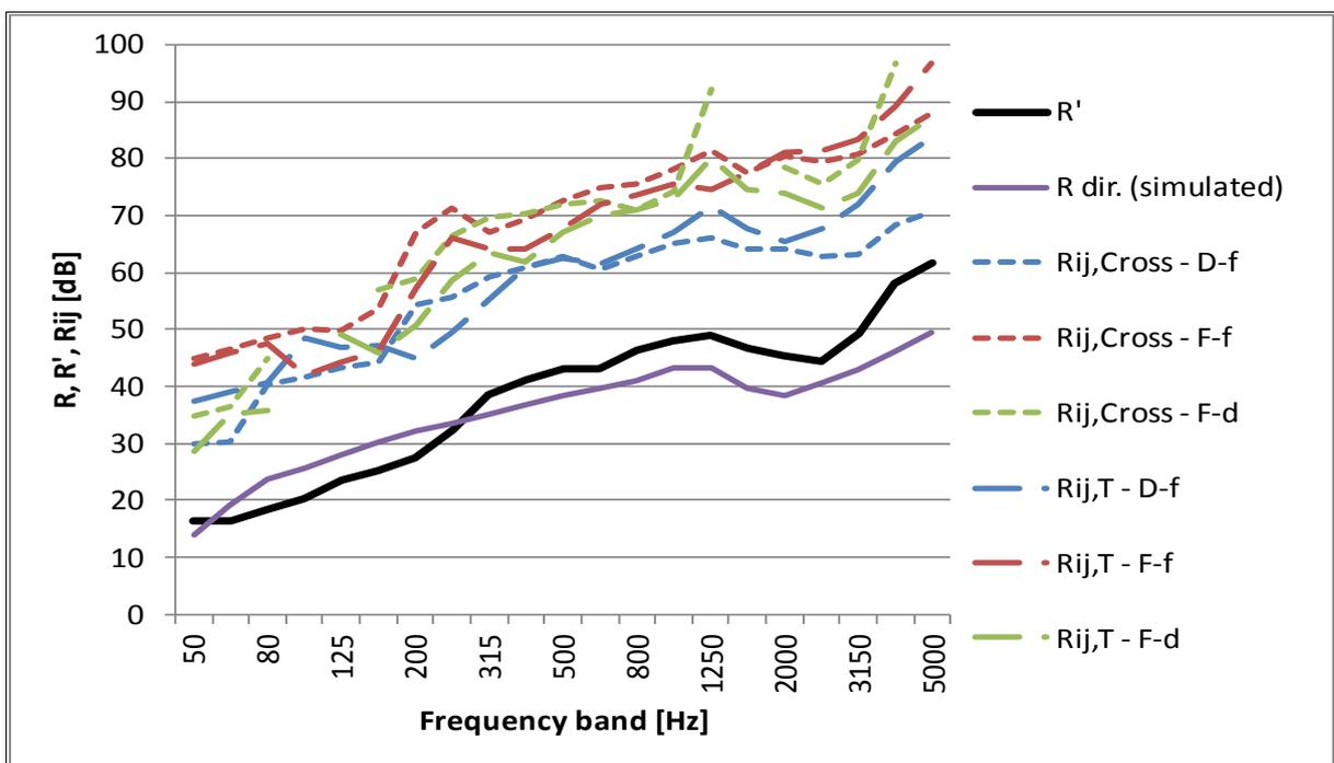
Figure e: Comparison of the (simulated) direct sound reduction index  $R$ , the measured overall sound reduction index  $R'$  and the measured flanking sound reduction indices  $R_{ij}$ .
