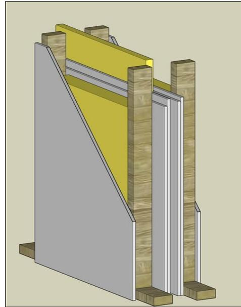
Composition: central cavity of 20 mm cavity filled with mineral wool 20 mm ca.  $16 \text{ kg/m}^3$  with symmetrically on both sides of the cavity (going from the inside towards the outside):: 1x12.5 mm fibre reinforced gypsum board \*\*\* 100x60 mm<sup>2</sup> studs, mineral wool 33  $\text{kg/m}^3$  100 mm \*\*\* 2x12.5 mm fibre reinforced gypsum board.
