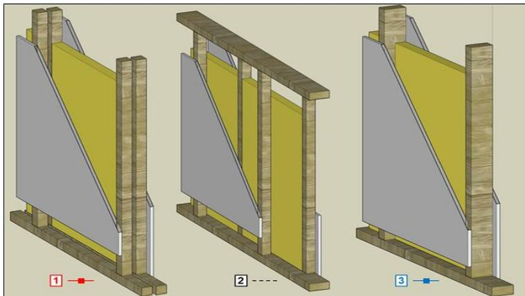
Figure 7c2 – DOUBLE WALLS: the more rigid connections are present, the bigger the losses in sound reduction index.
