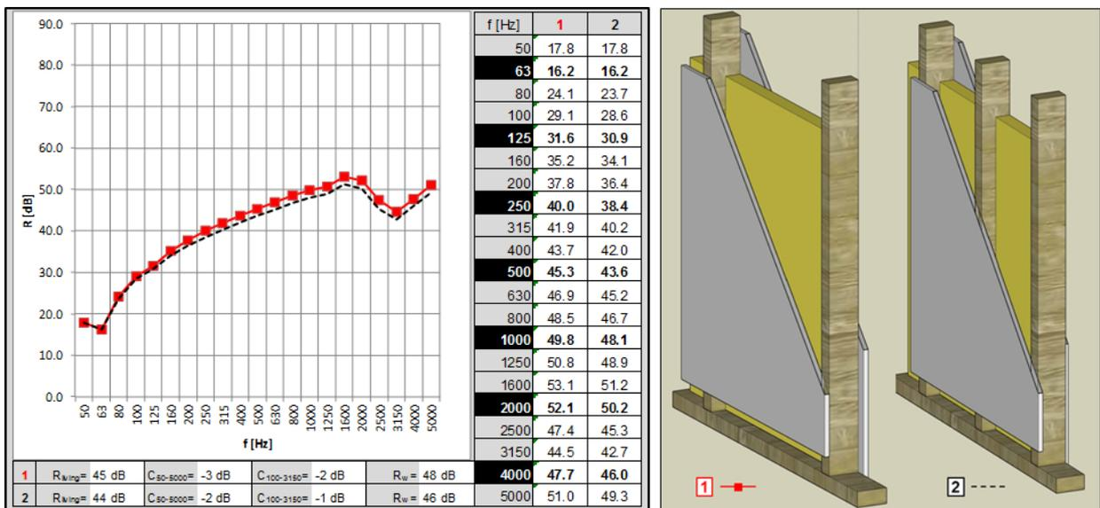
Figure 7f- DOUBLE WALLS: less rigid connections - for instance When the stud spacing increases, the number of rigid connections decreases which leads to a higher sound reduction index R. Graph 1 illustrates this effect for a stud spacing of 60 cm (o.c.), graph 2 shows the result for a stud spacing of 40 cm (o.c.). [Simulation with gypsum boards of 12.5 mm, mineral wool 5 cm, cavity width 10 cm, stud spacing o.c. 60 cm by INSUL 6.3 program of Marshall Day Acoustics].
