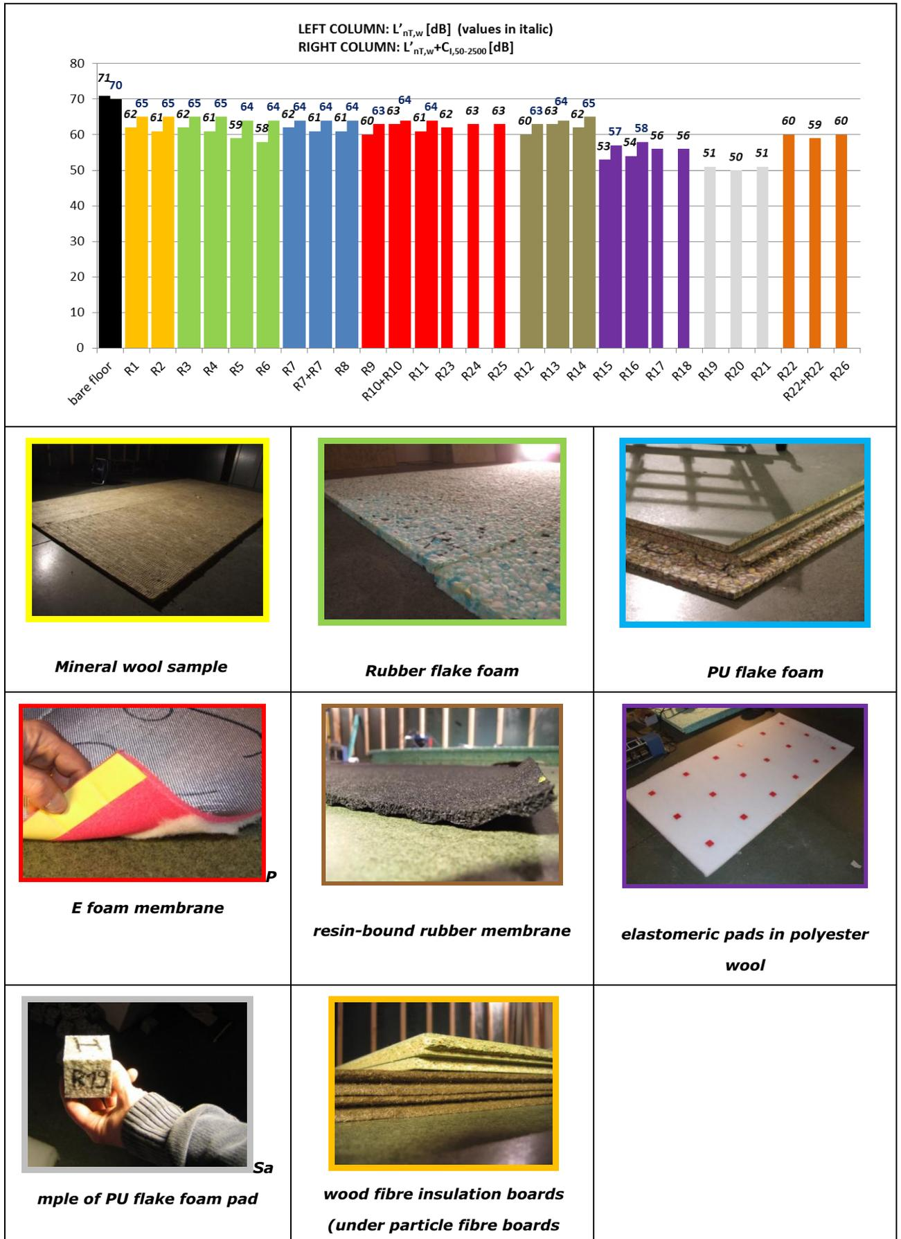
Chart 4:  $L'_{nT,w}$  results for different type of resilient layers combined loaded with a double layer particle boards (12 mm + 18 mm)
