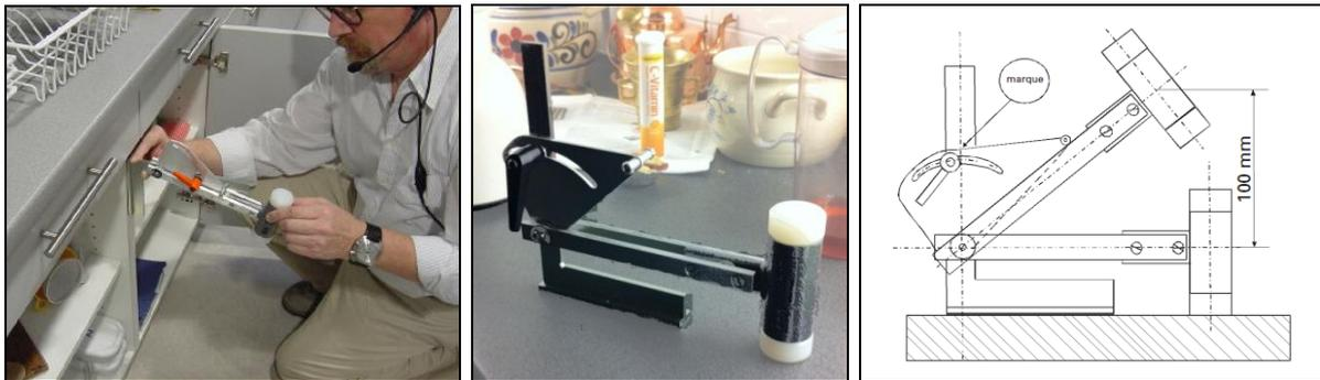
*Figure 22: Horizontal and vertical measurement with the pendulous hammer. This device was developed by the research institute EMPA in Switzerland. The aim was to evaluate impact noise of building service equipment in a simple and reproducible manner. The usage of the "pendulous hammer" is described in detail in the appendix B.3.5 of the SIA181:2006 standard.*
