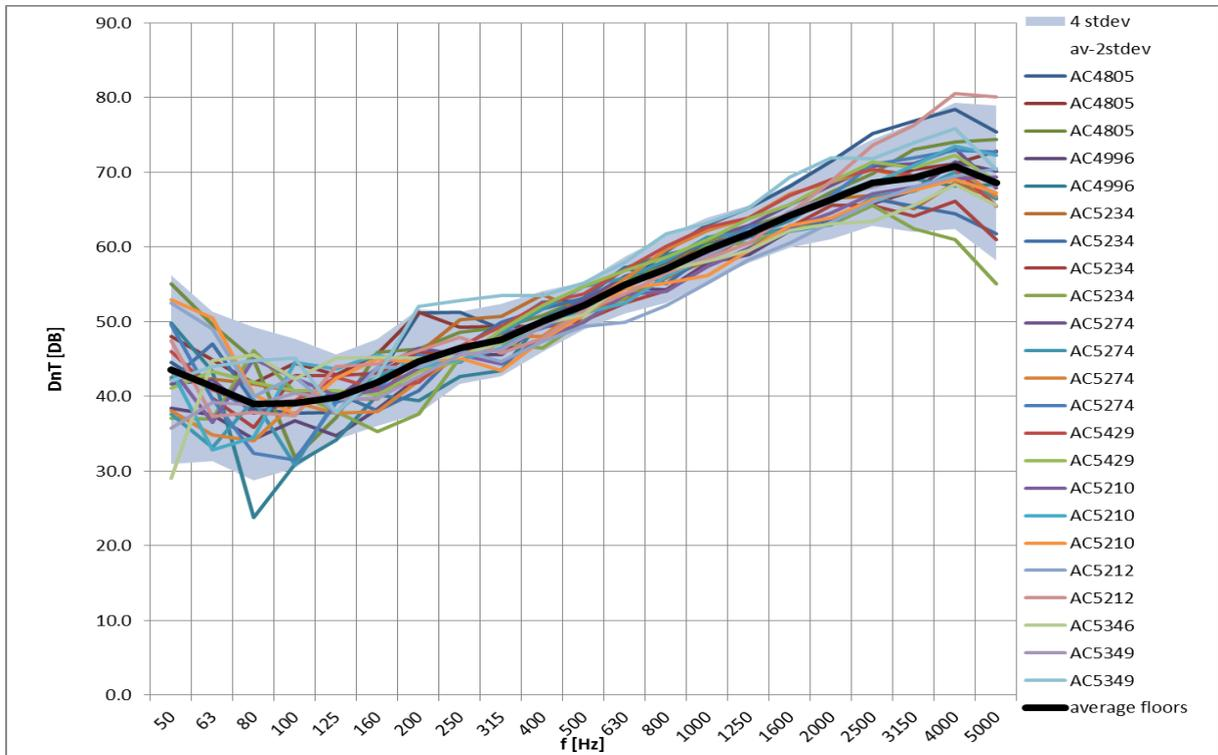
Graph 1: Different standardised level difference  $D_{nT}$  measured in situ on 23 well-executed traditional floating floors in Belgium. In the shaded zone, 95% of the measured values are situated.
