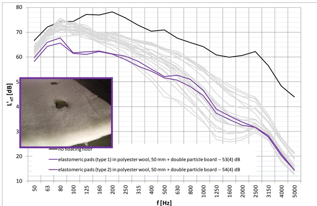
Chart 6: two different types of elastomeric pads tested in polyester wool
