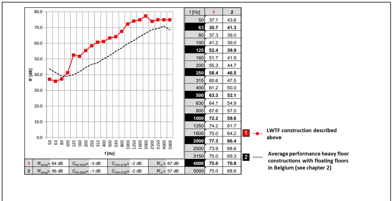
Figure 30: comparison of normalized impact sound levels and apparent sound reduction indices between an acoustically very well performing Finnish LWTF floor construction and the average result in heavy apartment constructions with floating floors (see discussion in section 2).
