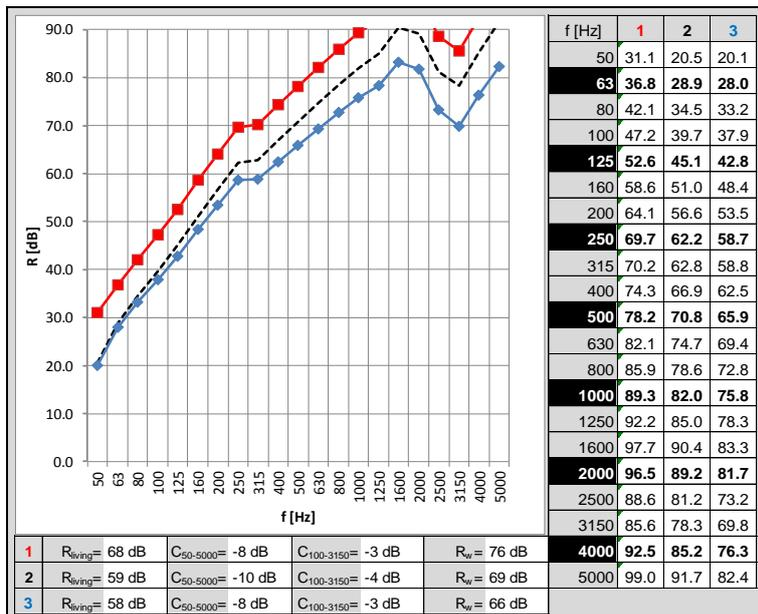
Figure 7g- DOUBLE WALLS: adding a supplementary thickness of acoustic absorbent (from graph 3 to graph 2) and more boards (from graph 2 to graph 1) allows for further increasing of the sound reduction index R. [Simulation with gypsum boards of 12.5 mm, mineral wool of 10 cm (case 3) and 20 cm (case 1 and 2), cavity width 20 cm,, stud spacing o.c. 60 cm by INSUL 6.3 program of Marshall Day Acoustics].
