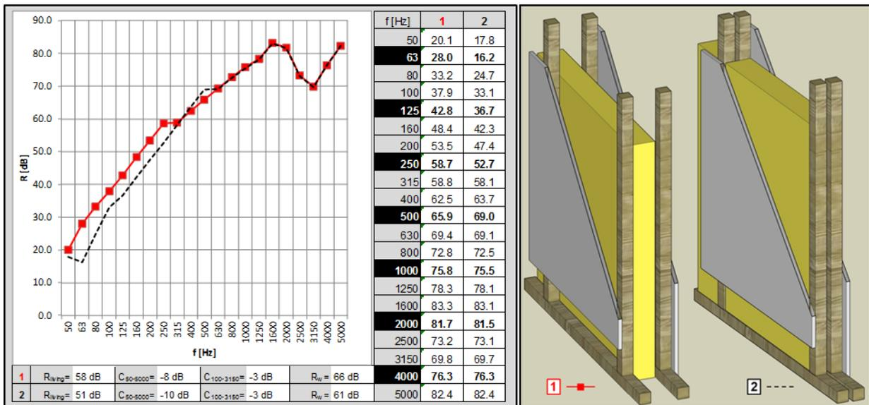
Figure 7f- DOUBLE WALLS: increasing the cavity width increases the sound insulation even in the very low frequencies. [Simulation with gypsum boards of 12.5 mm, mineral wool 10 cm, cavity width 10 cm for case 1 and 20 cm for case 2, stud spacing o.c. 60 cm by INSUL 6.3 program of Marshall Day Acoustics].
