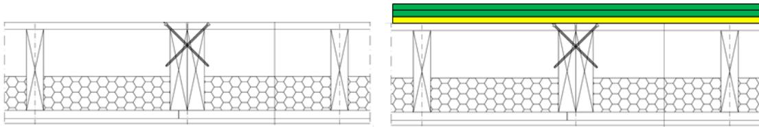
Figure 37: LEFT: construction of the reference timber floor. RIGHT: example of a floating floor on top of the reference floor.
