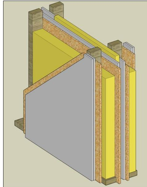
Composition: central cavity of 20 mm cavity filled with mineral wool 20 mm ca.  $16 \text{ kg/m}^3$  with symmetrically on both sides of the cavity (going from the inside towards the outside): 1x12.5 mm fibre reinforced gypsum board + 1x15 mm OSB \*\*\* 100x60 mm<sup>2</sup> studs, mineral wool  $33 \text{ kg/m}^3$  100 mm \*\*\* 1x15 mm OSB + 2x12.5 mm fibre reinforced gypsum board.
