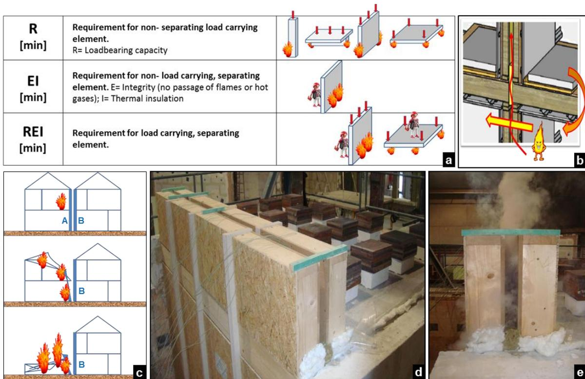
Figure 4: fire and the corresponding requirements have a major impact on how LWTF are conceived. This often leads to choices not very favourable for a good acoustic performance.
