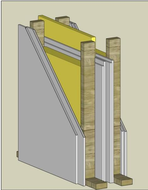
Composition: central cavity of 20 mm cavity filled with mineral wool 20 mm ca.  $16 \text{ kg/m}^3$  with symmetrically on both sides of the cavity (going from the inside towards the outside):: 2x12.5 mm fibre reinforced gypsum board \*\*\* 100x60 mm<sup>2</sup> studs, mineral wool 33  $\text{kg/m}^3$  100 mm \*\*\* 2x12.5 mm fibre reinforced gypsum board.
