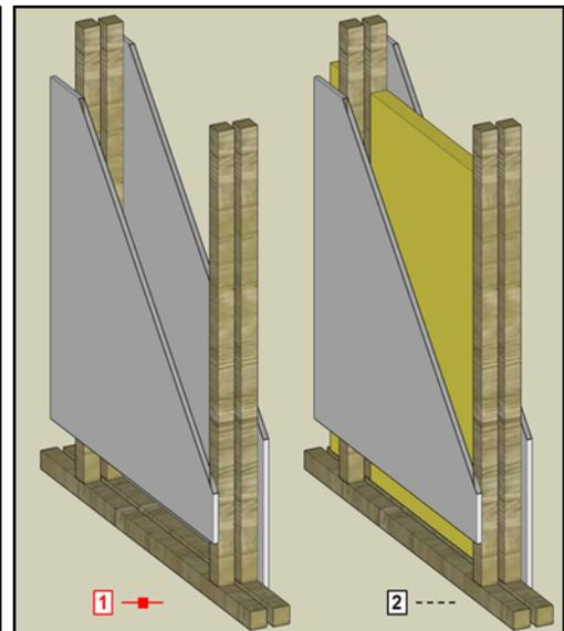
Figure 7d – DOUBLE WALLS: adding an acoustic absorbent increases dramatically the sound reduction index  $R$  when both wall portions are disconnected. [Simulation with gypsum boards of 12.5 mm, mineral wool 5 cm, cavity width 10 cm, stud spacing o.c. 60 cm by INSUL 6.3 program of Marshall Day Acoustics].
