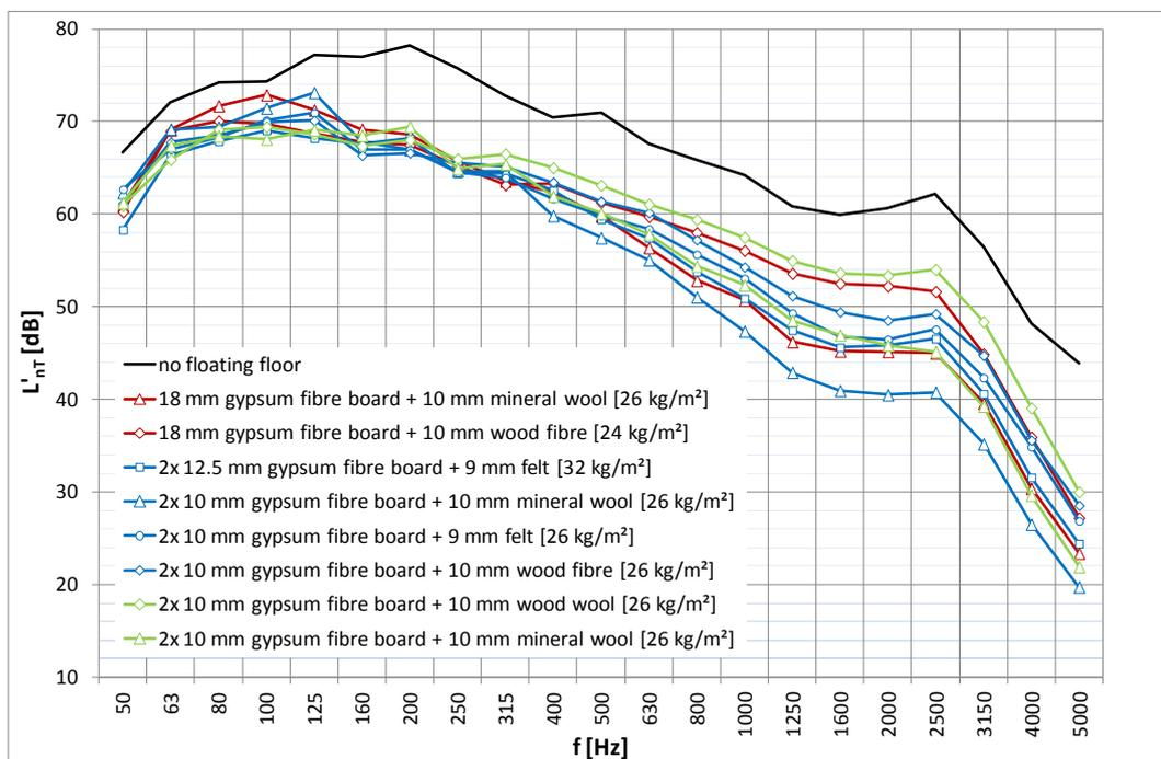
Chart 8: spectral comparison of different pre-assembled dry floating floor systems on reference floor
