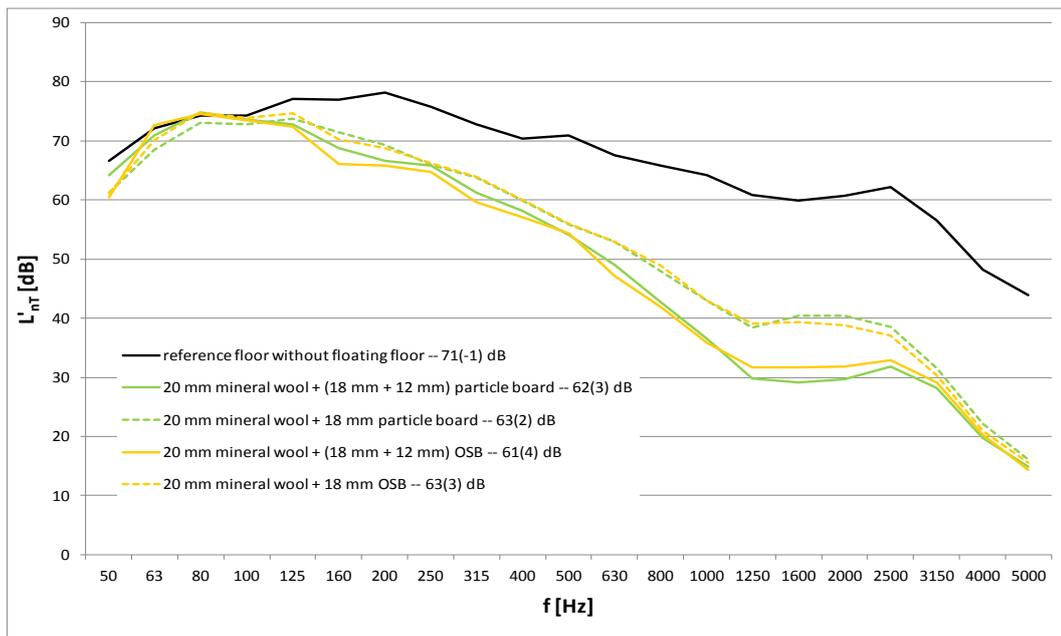
Chart 2: loading effect on 20 mm mineral wool for two different board types
