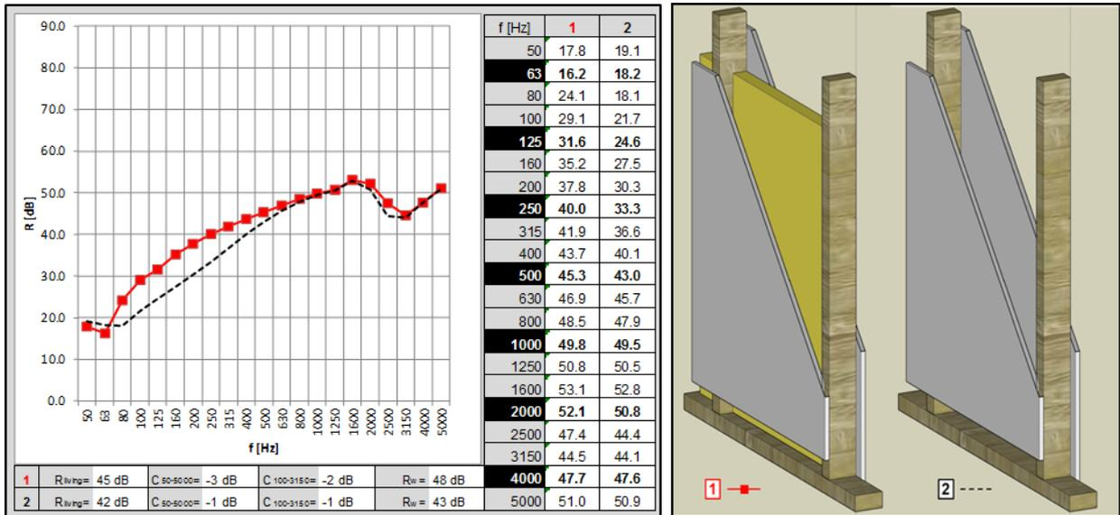
Figure 7e- DOUBLE WALLS: filling up the cavity with some acoustic absorbent can increase the sound reduction index even when there are rigid connections, though the effect is far less important than with disconnected walls (figure d). [Simulation with gypsum boards of 12.5 mm, mineral wool 5 cm, cavity width 10 cm, stud spacing o.c. 60 cm by INSUL 6.3 program of Marshall Day Acoustics].
