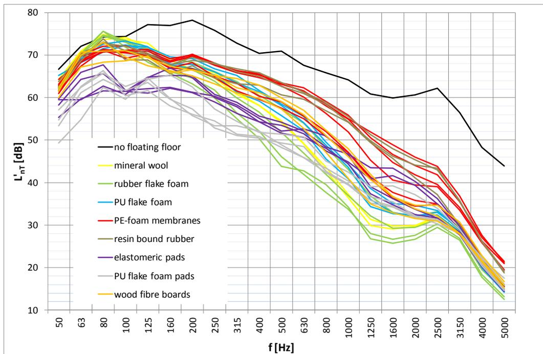
Chart 5: spectral comparison for different type of resilient layers tested under (12 mm + 18 mm) particle boards
