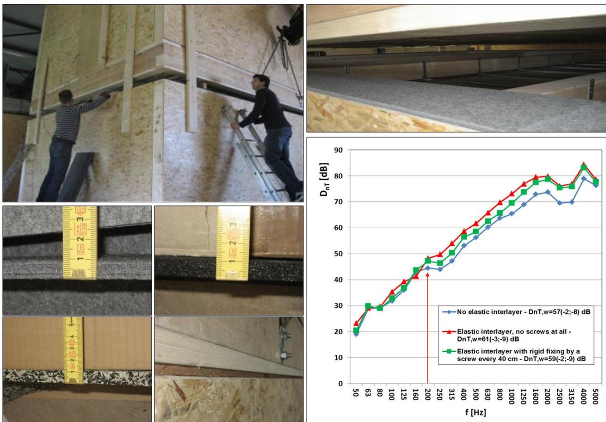
Figure 42 f: a pragmatic research examined the effect on the airborne standardised sound insulation  $D_{nT}$  of different linear and continuous elastic interlayers on the walls just below the floor of the room above. The system proved to be only effective above 200 Hz, showing no difference at all for the low frequencies.
