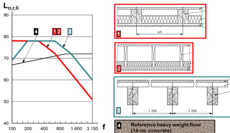
Figure 33: impact sound on reference floors as specified in EN ISO 10140-5. The improvement of the impact sound represents the difference between the impact sound measured directly on the reference floor and measured with the floating floor.
