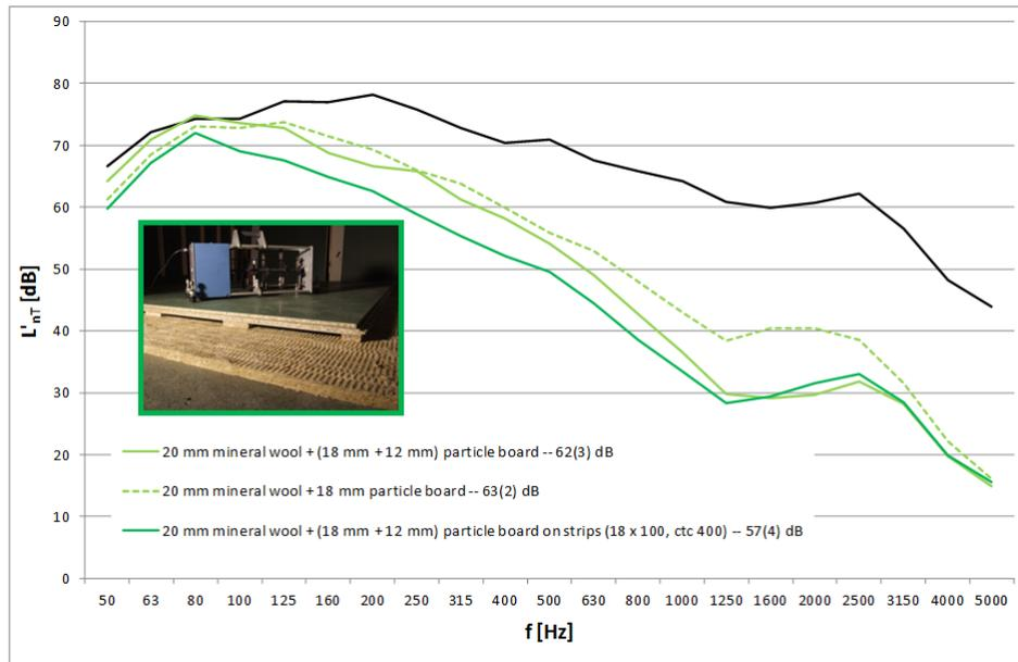
Chart 3: effect of concentrating load by means of wooden strips between boards and resilient layer
