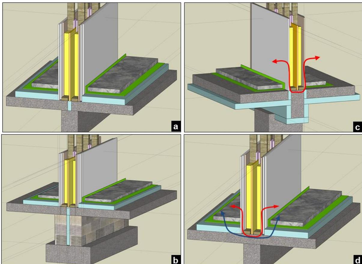
*Figure 26: some possible foundations and junctions with the party wall. The use of floating floors is everywhere recommended to avoid impact sound. In figures 'c' and 'd' the maximum possible sound insulation that can be obtained with the party wall will not be attained due to a connecting path between both wall portions via the concrete slab/ beam.*
