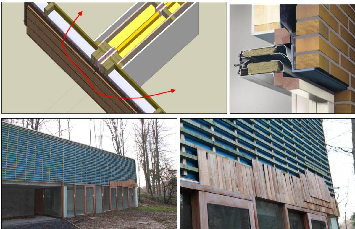
*Figure 29: transmission path 2 when the sound façade insulation is low (rigid thermal insulation with closed cells, cladding, cedar tiles,...). Ventilation grids should have a minimal acoustic sound insulation to avoid indirect sound transmission*
