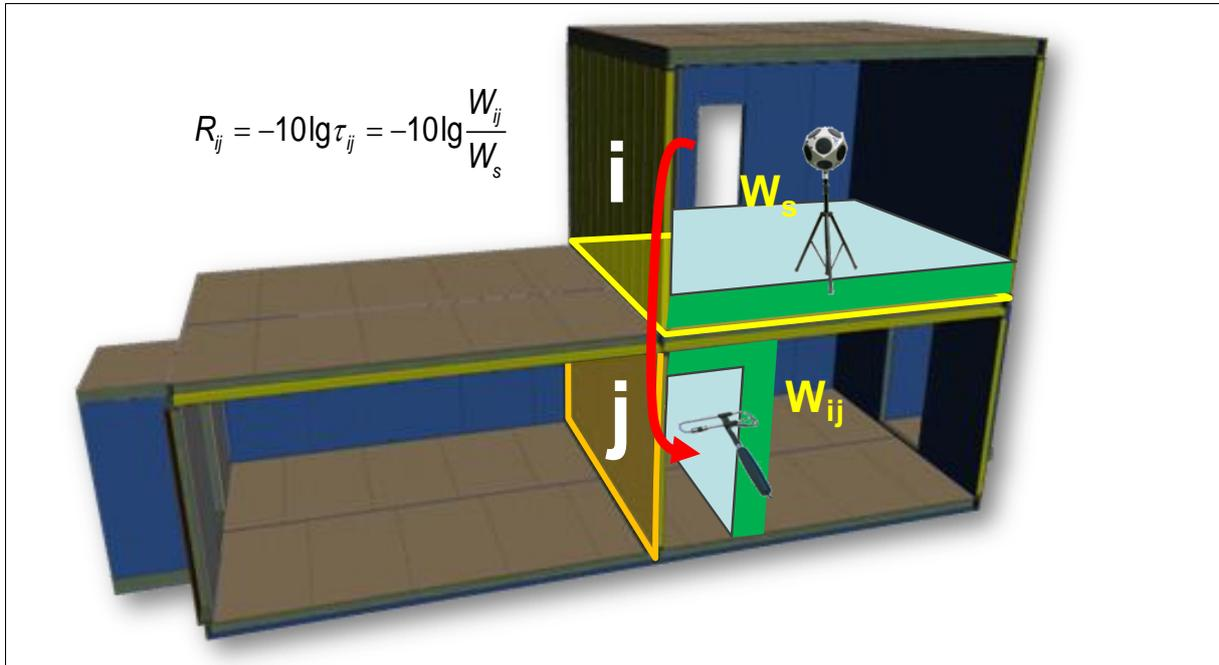
Figure 45 b: Test setup example for measuring the flanking sound reduction index
