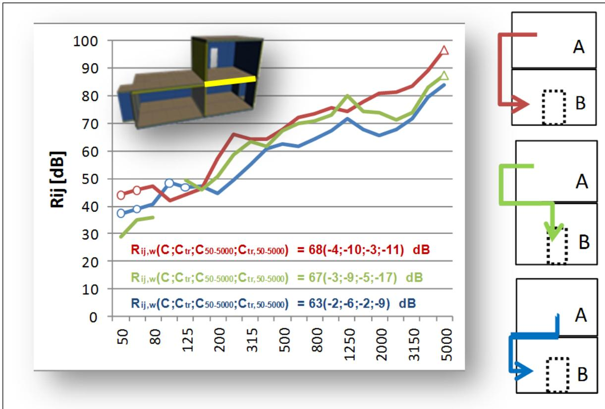
Figure 45 d: Measured flanking sound reduction indices on the T junction for the 3 paths Ff, Fd and Df. Values indicated with a triangle are minimal values, whereas values indicated with a circle are interpolated or extrapolated values (-5 dB/octave going down at low frequencies).
