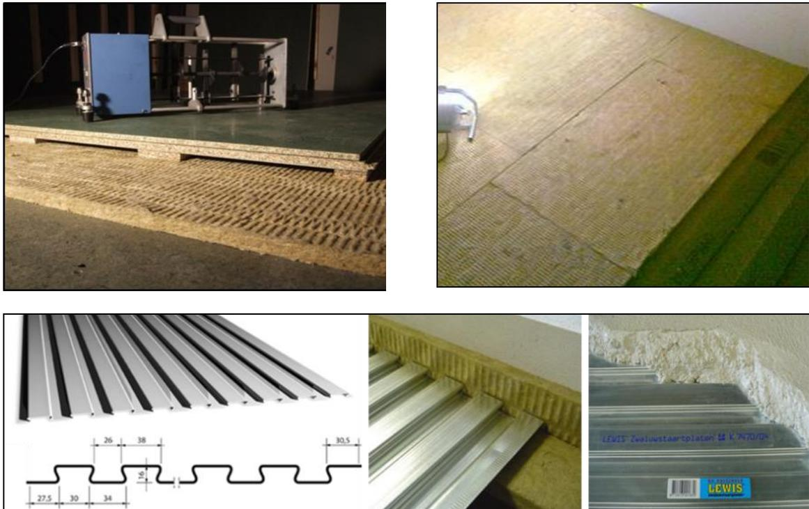
Figure 35: illustrations of floating floors SYSTEM 2 solutions based upon the principle of concentrating mass carrying line-wise on an elastic interlayer.
