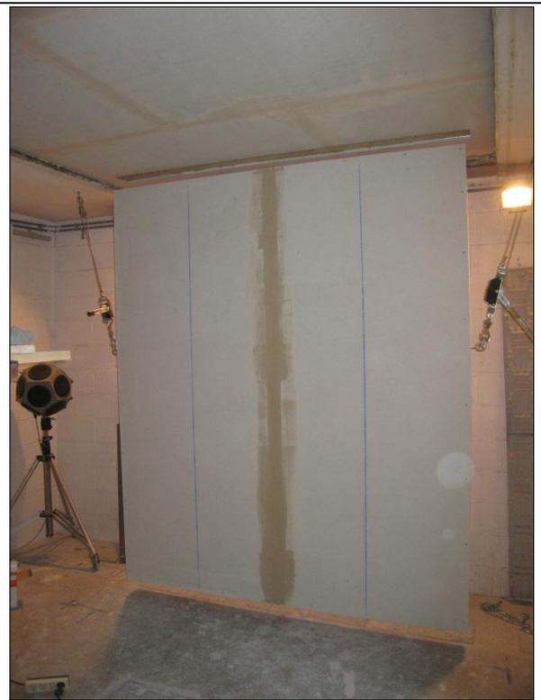
Figure e: T-junction with the studwall rigidly fixed on top of and below the floor
