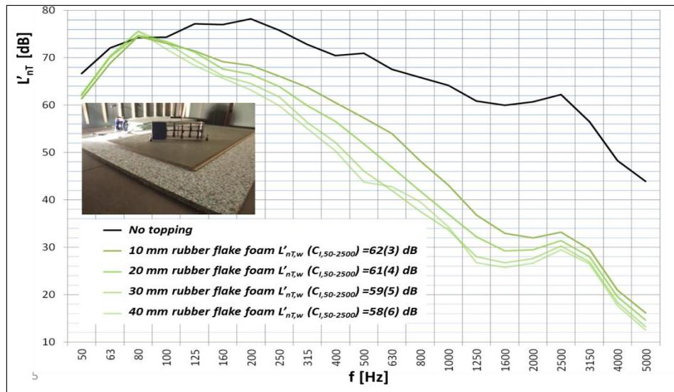
Chart 10: influence of the thickness of the elastic interlayer. Increasing the thickness of the rubber flake foam diminishes its stiffness. Doubling the thickness from 10 mm to 20 mm reduces the stiffness with 2; 40 mm thick foam only has a quarter of the stiffness of 10 mm foam. One would expect a downwards shift of the mass-spring-mass resonance with diminishing stiffness, but this was not noticeable in the measurements.
