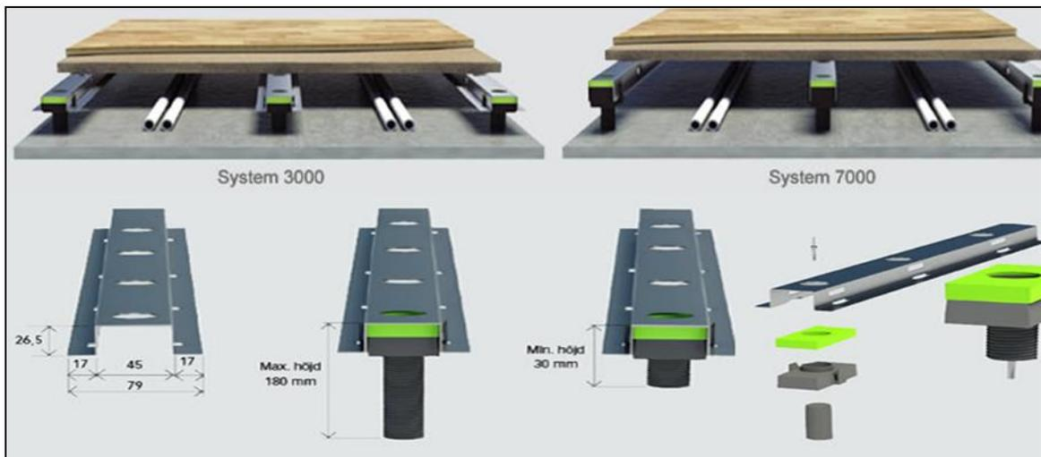
Figure 36: illustrations of SYSTEM 3-solutions based upon the principle of concentrating mass carrying point-wise on elastic pads. Pictures c is from from CDM company (pads and iso-lats) see [www.cdm.be](http://www.cdm.be). Pictures d is from Granab Subfloorsystems [www.granab.se](http://www.granab.se)
