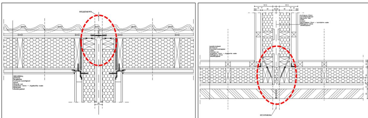
Figure 25: the decoupling should also be respected at the borders of the party wall (junction with the roof to the left, junction with the façade to the right)
