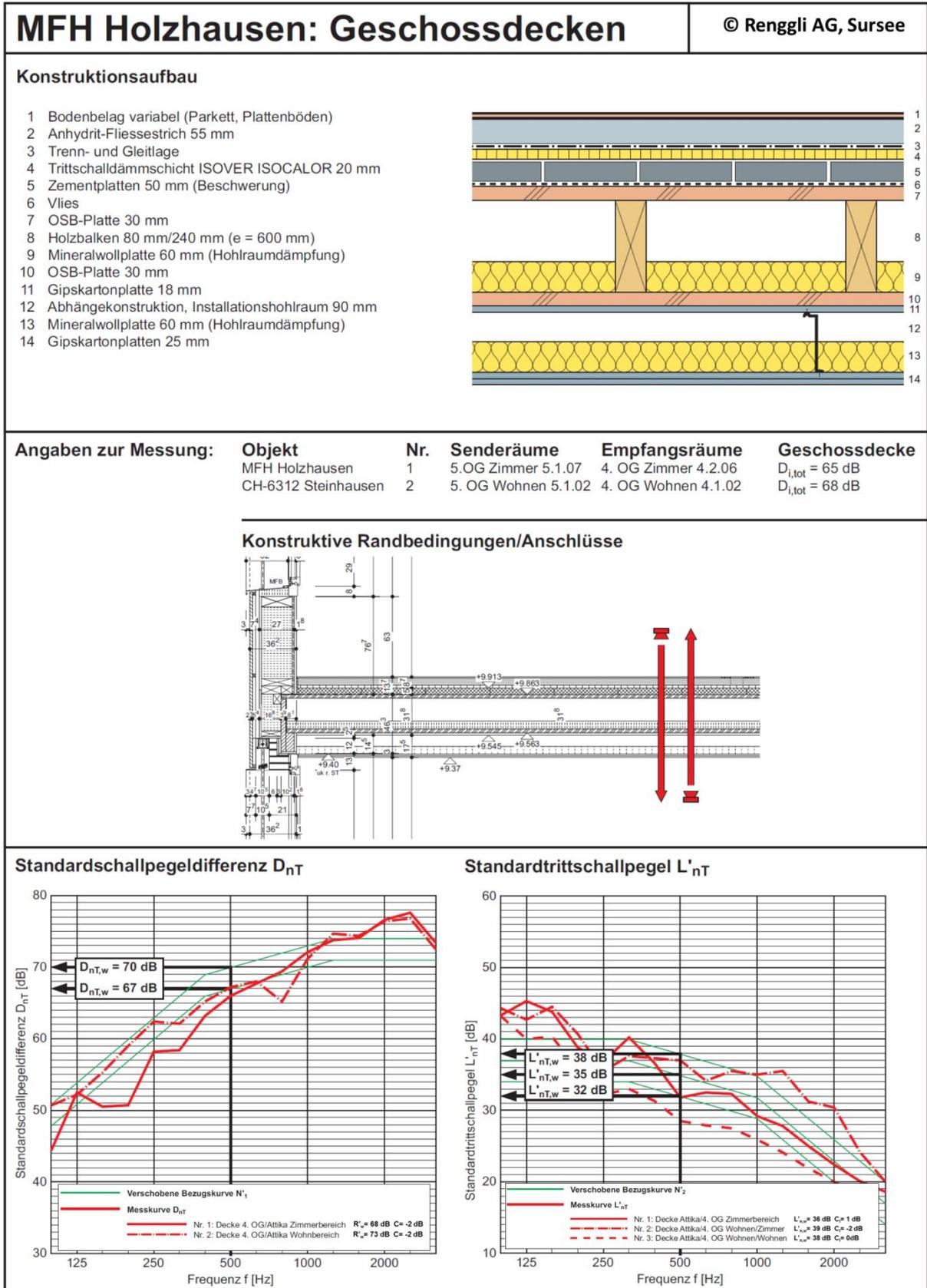
Figure 31: floor construction in the first 6 floors high LWTF project in Steinhausen, Switzerland (MFZ Holzhausen, © Renggli AG, Sursee).
