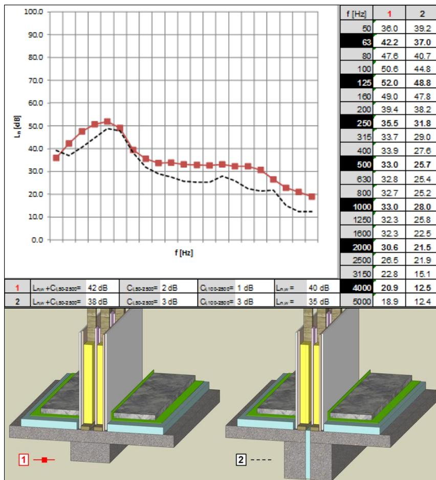
Figure 27: comparison avec the impact sound insulation with well executed floating floors. Both results are excellent, but the interrupted concrete slabs have a 4 dB better performance and offers some additional 'insurance' for the case when something goes wrong with the floating floor. (Measurements BBRI-MBS RE Hechtel-Eksel liv23liv21 for case 2 and liv19liv21 for case 1)
