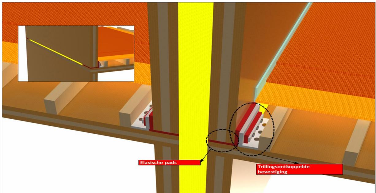
Figure 42 h: the use of elastic pads, creating only discontinuous elastic contact points every 150 cm appears to have a better effect in the low frequencies (BBRI-La Maison Idéale Project).
