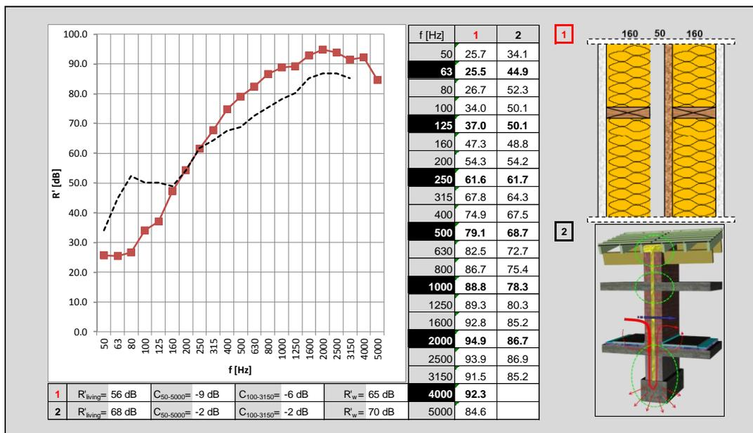
Figure 6: comparison between the sound insulation  $R'$  of two compartment walls: (1) of a lightweight timber frame wall; (2) of a traditional tie-less brick construction as a typical compartment wall between two terraced houses or apartments (reference graph)
