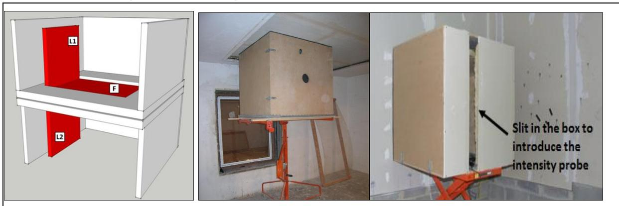
Figure 43: LEFT: laboratory setup; MIDDLE and RIGHT: a semi-anechoic box (protecting against the noise influence from the acoustic hall) was used to measure the radiated sound of the wall via the intensity technique
