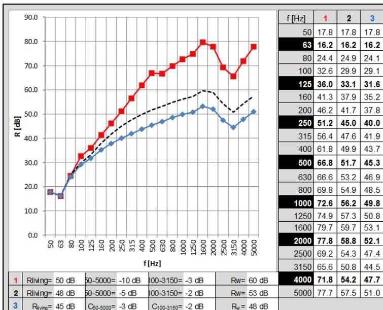
Figure 7c1 - Graph 1: completely decoupled double wall / Graph 2: staggered constructions only connected on top and below the wall. / Graph 3: studs connect both wall portions. Coincidence dips are marked by 'c', the mass-spring-mass resonance dip is marked by 'r'.
