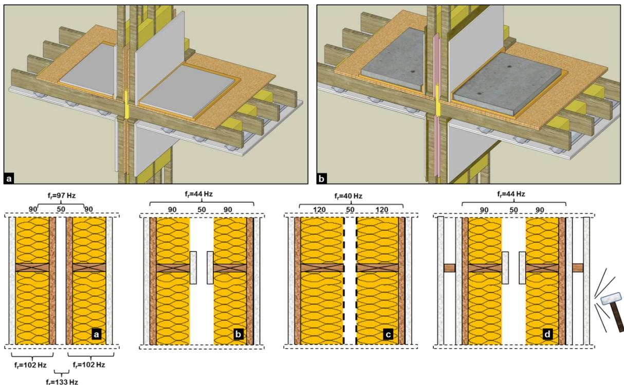
Figure 18: (a) traditional solution; (b) and (c) creating large cavities allows shifting the mass-spring-mass resonance frequency to the very low frequencies increasing considerably the low frequency sound insulation. Fire requirements impose special measures to be undertaken; (d) technical linings help to diminish sound coming from cupboards, tapping against the wall...
