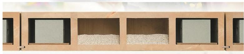
**Figure:** the Swiss company 'Lignatur' has some specific solutions for compartment floors. Box and surface elements constitute the load-bearing floor. Different types of toppings allow attaining a wide variety of acoustic performances. The picture down left shows a highly damped solution with dry concrete blocks and grit fillings, optimizing the low frequency sound insulation and acoustic comfort (damping the modal peaks and resonances).
