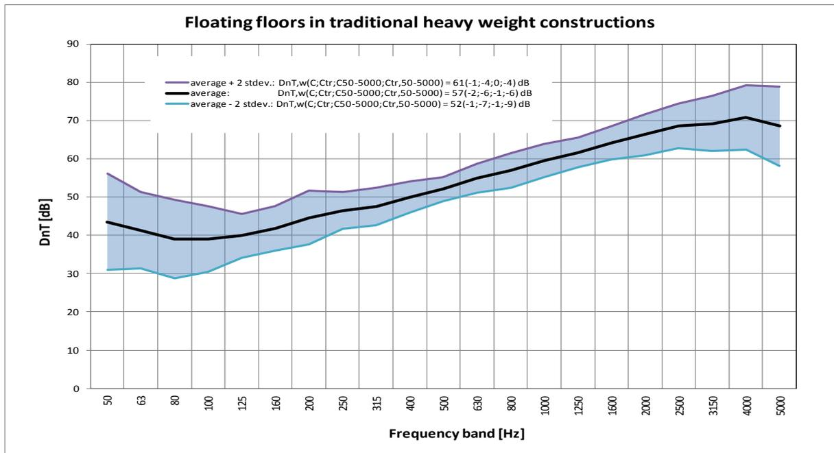
Graph 3: Average spectrum of the standardised level difference  $D_{nT}$  measured in situ on 23 well-executed traditional floating floors in Belgium. 95% of the measured values are situated inside the shaded zone.
