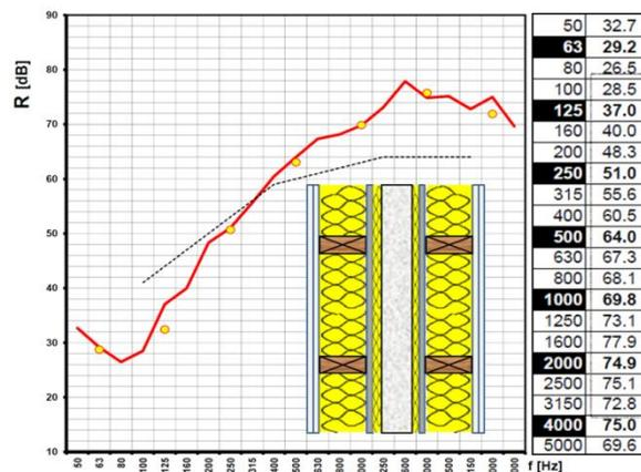
Figure 9: construction of the party wall composed of 5 cm gas concrete completed symmetrically on both sides with 20 mm glass wool, a cement board of 9 mm, studs of 90 mm x 40 mm and a cavity filled with mineral wool and finally 2 x 12.5 mm gypsum boards.
