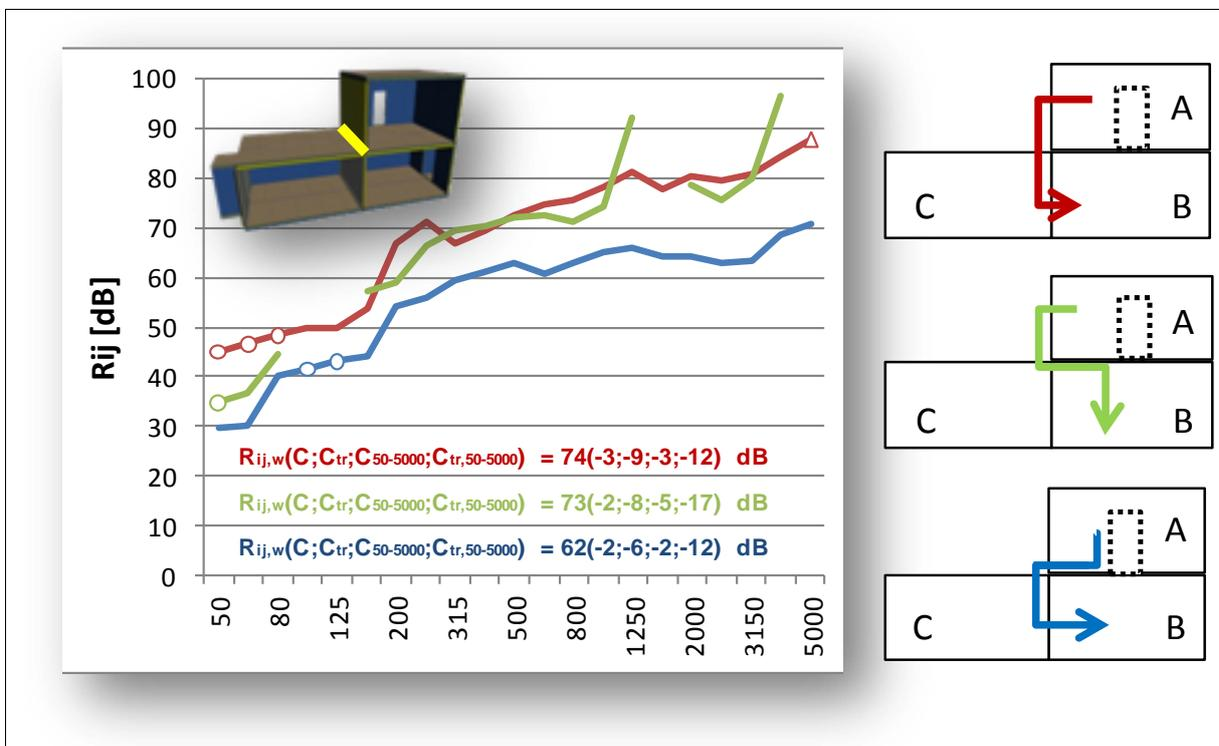
Figure 45 c: Measured flanking sound reduction indices on the cross junction for the 3 paths Ff, Fd and Df. Values indicated with a triangle are minimal values, whereas values indicated with a circle are interpolated or extrapolated values (-5 dB/octave going down at low frequencies).
