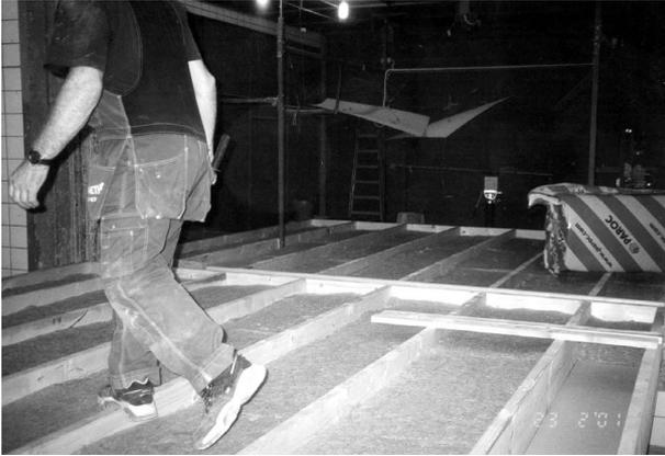
Figure 1.3: A lightweight wall and a lightweight floor construction adjoining it were built in the sound-transmission laboratory at LTH, Lund. Photo: Lars-Göran Sjökvist.
