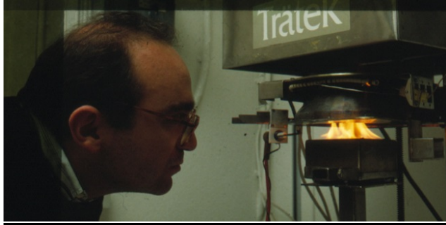
Figure 6. ISO 5660, Cone calorimeter, with sample size 100 x 100 mm. Used for product development and for verifying the reaction to fire performance after weathering.
