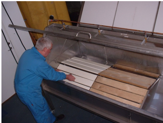
Figure 7. Accelerated ageing of FRT wood panels according to NT FIRE 053 and CEN/TS 15912 (with box open).
