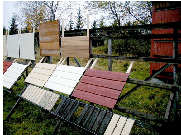
Figure 8. Natural field weathering of FRT wood panels exposed both vertically (90°) and at 45° slope outside Stockholm, Sweden.
