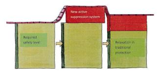
Figure 3: Principle for fire safety design by sprinklers: Increased fire safety by installation of sprinklers may lead to relaxations in the passive fire protection features, and still fulfil the same or higher safety level [23].
