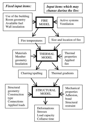
Figure 2: Flow chart for predicting structural fire performance [6]
