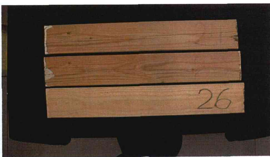
Figure 6.1 Colour changes in panels exposed to UV light or not.
