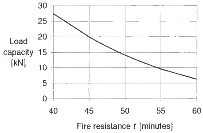
Figure 4.9: Example of relationship between load bearing capacity of stud and fire resistance (time to failure)
