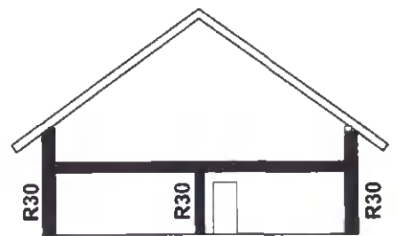
Fire resistance – requirement levels
