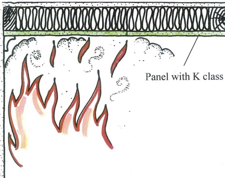
Figure 1. Principle for Testing Fire Protection Ability According to EN 14135.
