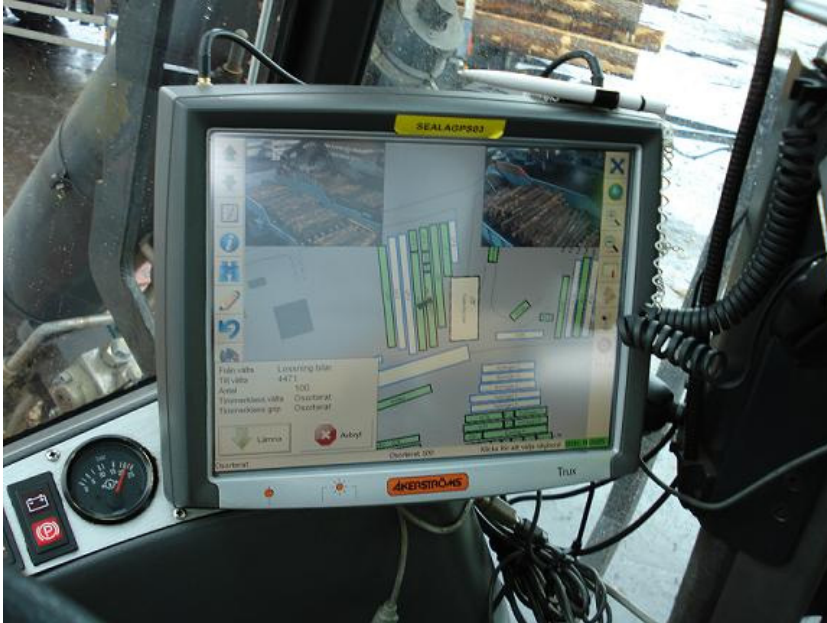
Figure 5.16 GPS Timber decision support system setup in a log stacker cab.
