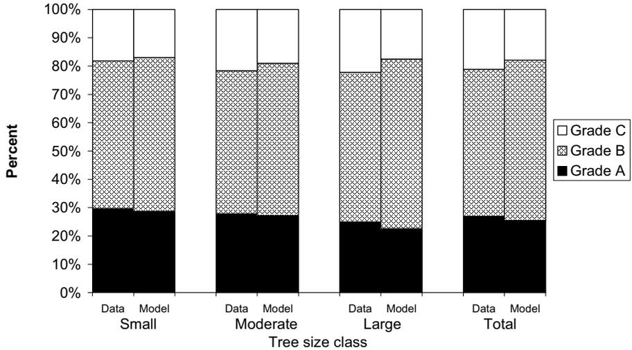
**Fig. 7.** Timber grade distribution by tree size class using tree model and empirical measurement data respectively.
