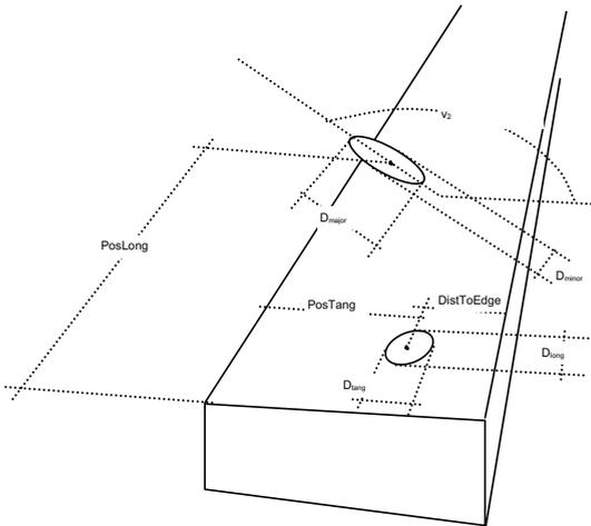
**Fig. 17.** Notations used when calculating knot diameters.
