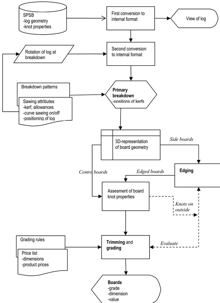
**Fig. 1.** Flow of operations in Saw2003 from loading raw log description from Swedish Pine Stem Bank (SPSB) through conversion to final products.
