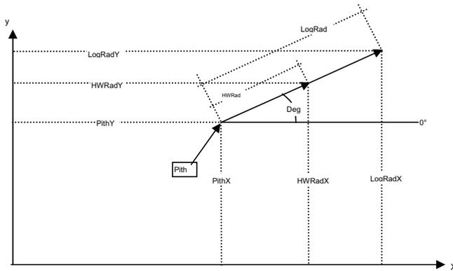
**Fig. 3.** Cross-section of log is represented with polar coordinates of heart wood radius (HWRad) and surface radius (LogRad) originating from pith. Coordinates are converted to rectangular coordinates.
