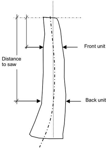
**Fig. 12.** Principle of curve sawing at second saw. The curve crosses the straight log centre line at centering units when the offset is set to 0.
