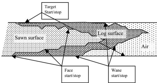
**Fig. 14.** Representation board side. Board side is built up by an array of 1D-profiles which define start and stop coordinates of sawn surface, log surface and targets.
