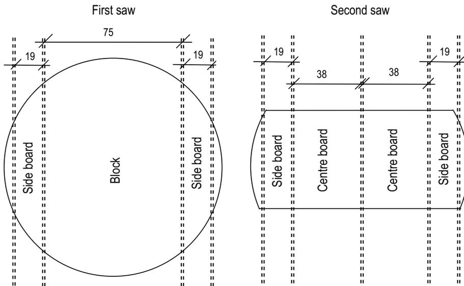
**Figure 3.** Illustration of sawing patterns (using the pattern for the smallest log of Table 3 as an example) used with cant sawing.
