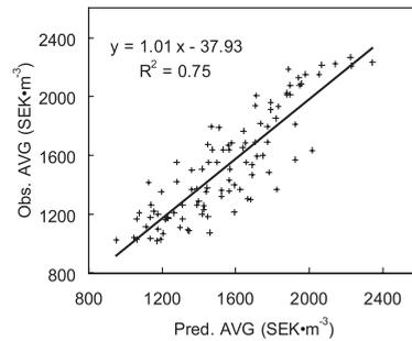
Fig. 3. Predicted and observed average board value (AVG) for the independent test set of 100 logs using model M:3D-X.
