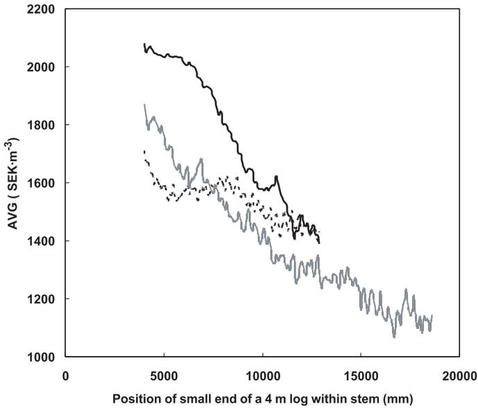
Fig. 4. Average board value (AVG) predicted with model M:3D on a 4 m log at different positions within the stem. Example with three stems.
