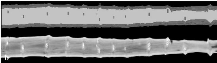
**Fig. 6.** Board reconstructed from simulated sawing based on parametrical description of a log (a) and corresponding section of the CT image stack (b). N.B. Horizontal and vertical scaling are not equal.
