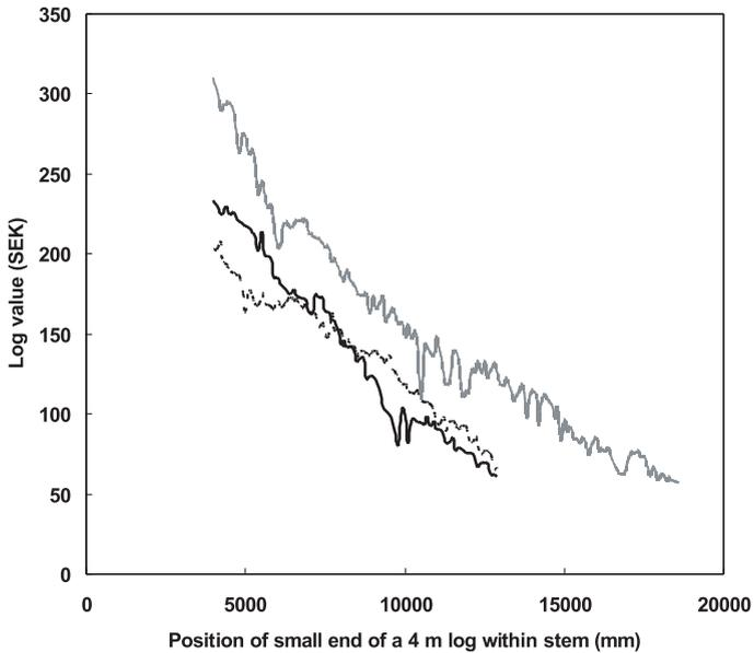
Fig. 5. Gross value of a 4 m log at different positions within the stem estimated by combining predictions of board values with model M:3D and volume yield predicted with the sawmill simulator software Saw2003 and adding the value of byproducts. Example with three stems.
