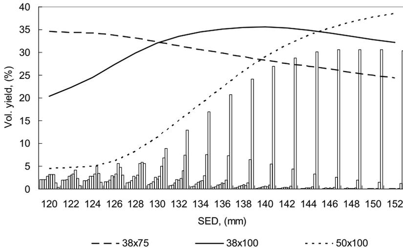
**Figure 2.** Predicted volume yield length distribution of 38- x 100-mm boards yielded from 4300-mm-long logs with varying small-end diameter. Yield is expressed as proportion of log volume. In each presented 2-mm-wide log class, the leftmost bar represents boards 1800 mm long, and succeeding bars show boards with a 300-mm length increment up to the rightmost bar representing 4200-mm-long boards. Lines show total volume yield for three competing dimensions.
