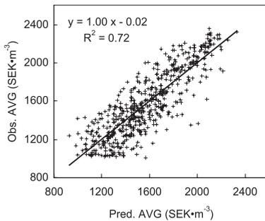
Fig. 2. Predicted and observed average board value (AVG) for the training set of 515 logs using model M:3D-X.
