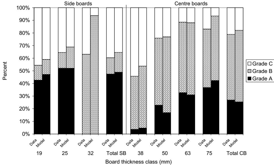
**Figure 8.** Lumber grade distribution by board thickness class using tree model and empirical measurement data respectively.
