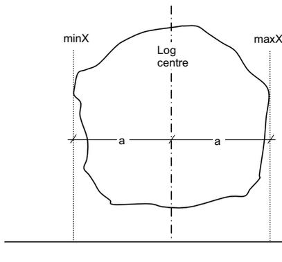
**Fig. 11.** Principle of determining the centre position of a log cross-section at first saw.
