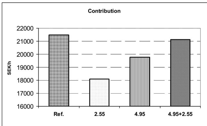
**Fig. 12.** Contribution per hour calculated by combining product flow with product value in four bucking alternatives.
