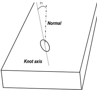
**Fig. 16.** Cylindrical diameter of knot at point of intersection is projected to board face.
