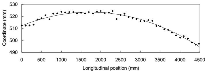
**Fig. 9.** Regression line of centre of gravity at longitudinal positions within log. Example with log 1,1,1 from SPSB and rotated crook upwards.
