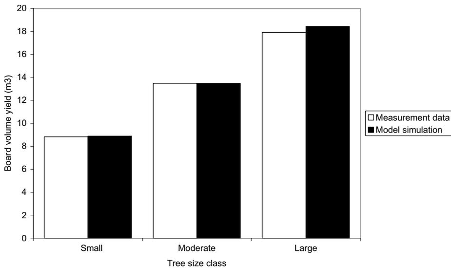
**Figure 5.** Lumber volume yield by tree size class using tree model and empirical measurement data respectively.
