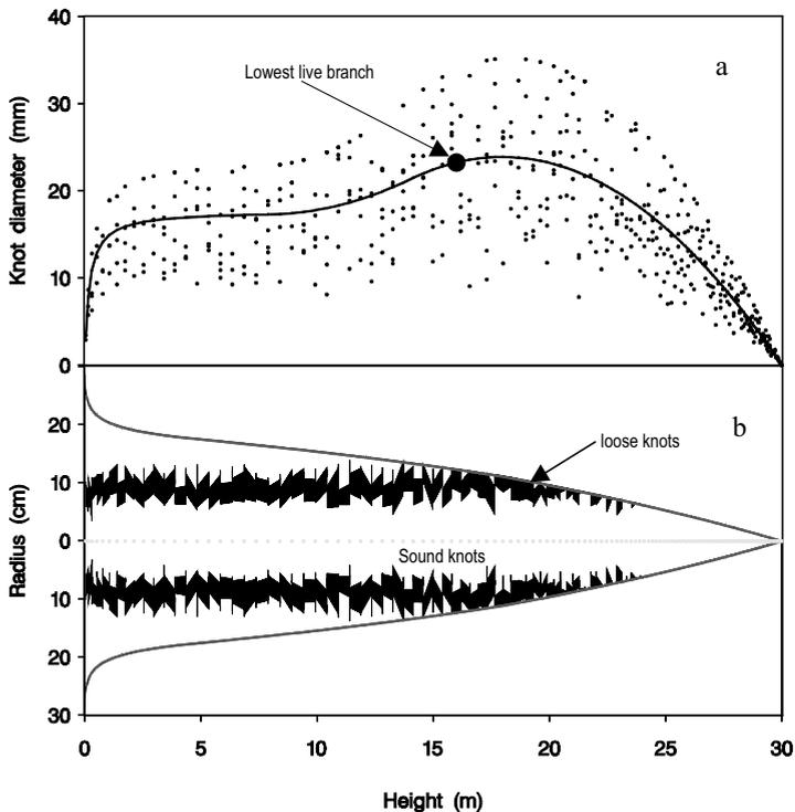
**Figure 4.** Illustration of simulated knot diameter, knot type, whorl location and stem taper.
