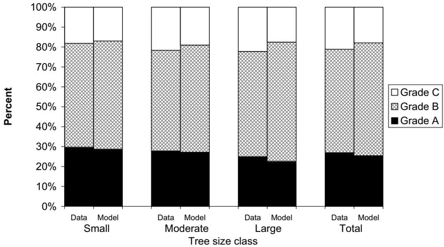
**Figure 6.** Lumber grade distribution by tree size class using tree model and empirical measurement data respectively.
