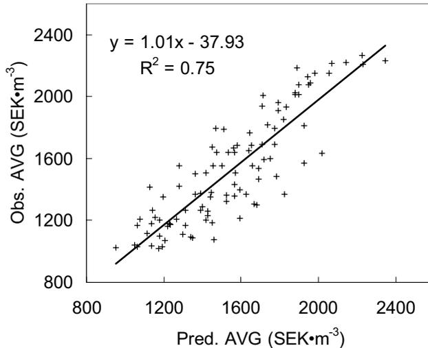
**Fig. 8.** Predicted and observed average board value (AVG) for the independent test set of 100 logs using model M:3D-X.
