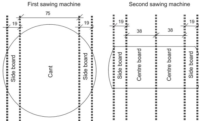
Fig. 1. Cant sawing. The first sawing machine cuts the log into side boards and a cant. The cant is then rotated by 90 degrees and cut by the second sawing machine into side boards and centre boards. Side boards are further processed by edging and trimming, while trimming is the only operation on centre boards. Example with the first sawing pattern listed in Table 1.
