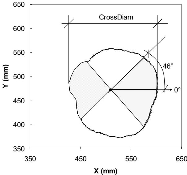
**Fig. 5.** Illustration of the *CrossDiam* measure. Example with search for the maximum extension in direction  $0^\circ$ . Search is done within shadowed areas.
