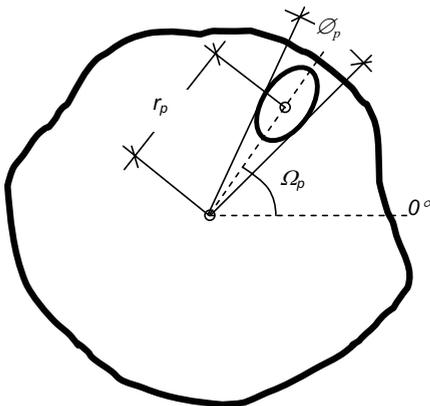
Fig. 6. Knot geometry notation, projection to a cross-section
