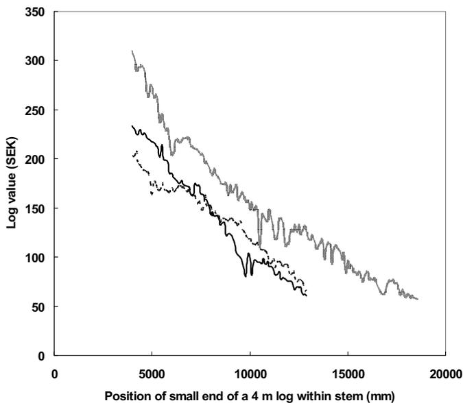
**Fig. 10.** Gross value of a 4-m log at different positions within stem estimated by combining predictions of board values with model M:3D and volume yield predicted with the saw mill simulator software Saw2003 and adding the value of byproducts, example with three stems.
