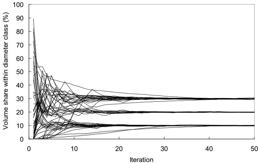
**Figure 7.** Evolution of volume shares of sawlogs within diameter classes using adaptive log prices for production control in bucking. Targeted shares were 10% 3700-mm-long logs, 30% 4300 mm, 20% 4600 mm, 30% 4900 and 10% 5200 mm within each 20-mm-wide diameter class.
