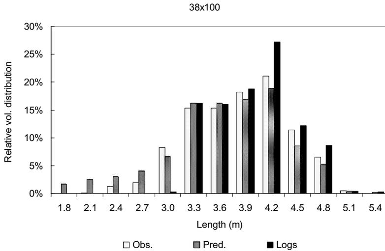
**Figure 4.** Sawmill's distribution of logs by length classes within diameters 127 mm to 142 mm SED and predicted and observed length distribution of 38- x 100-mm boards yielded from sawing the same logs. Actual log lengths within a length class were 100 mm to 399 mm longer, while logs used for simulation were 100 mm longer than length class shown.
