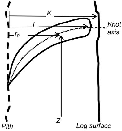
Fig. 7. Knot geometry notation, projection to a radial section.
