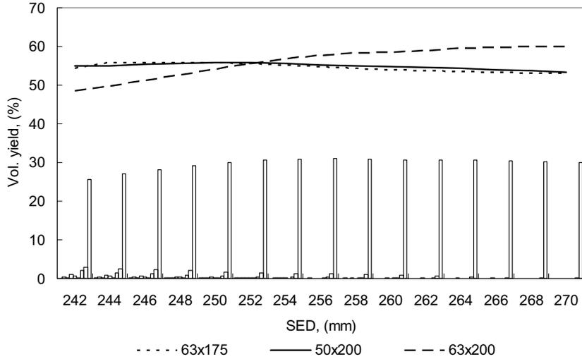
**Figure 3.** Predicted volume yield length distribution of 50- x 200-mm boards yielded from 4300-mm-long logs with varying small-end diameter. Yield is expressed as proportion of log volume. In each presented 2-mm-wide log class, the leftmost bar represents boards 1800 mm long and succeeding bars shows boards with a 300-mm length increment up to the rightmost bar representing 4200-mm-long boards. Lines show total volume yield for three competing dimensions.
