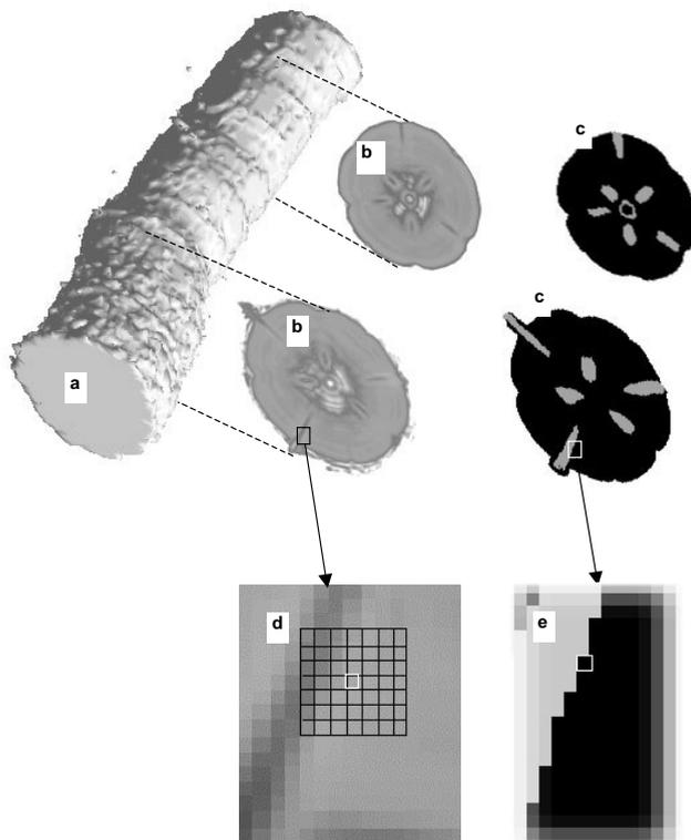
**Fig. 2.** Schematic description of the ANN method. From a log scanned with CT (a), digital images of transverse sections containing whorls were chosen (b). Grey-scale values of a squared window with the targeted pixel in the centre are fed to the ANN as input (d). During the training stage the desired output (e) is given by manually classified duplicates (c). Iterating through the images, the prediction error is minimised and the trained ANN can be used as a pixelwise classifier.
