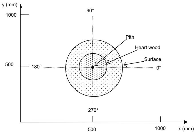
**Fig. 4.** Representation of cross-section of log, viewed from top-end towards butt-end. Log is fitted within a 1000 mm  $\times$  1000 mm coordinate system and translated so that pith at both log ends is positioned at (500, 500).
