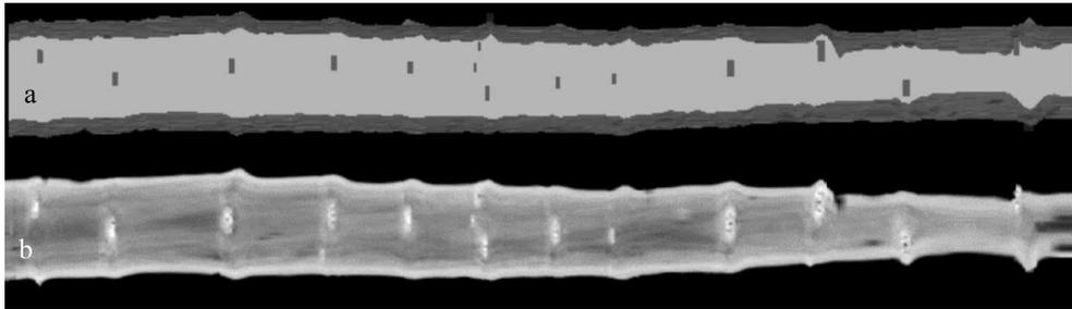
Fig. 7. Board reconstructed from simulated sawing based on parametric description of a log (a) and corresponding section of the computed tomographic image stack (b). NB. Horizontal and vertical scales are not equal.
