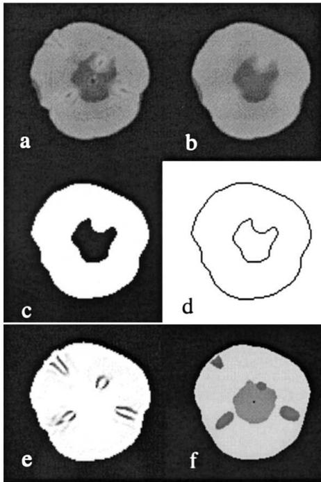
Fig. 2. Images of a log cross-section at different stages of parameter extraction: (a) original computed tomographic image; (b) after application of a  $7 \times 7$  median filter on image (a); (c) thresholded binary of image (b); (d) boundary outline of image (c); (e) knot borders predicted by the artificial neural network; (f) cross-section as reconstructed from parametric description.
