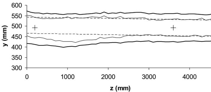
**Fig. 18.** Outer face as made up of the array of SideProfile. Thick solid lines are wane\_start and wane\_stop. Thin solid lines are face\_start and face\_stop. Dashed lines are the best edging solution from table 2. Plus signs are the end-points from which possible edging patterns are built.
