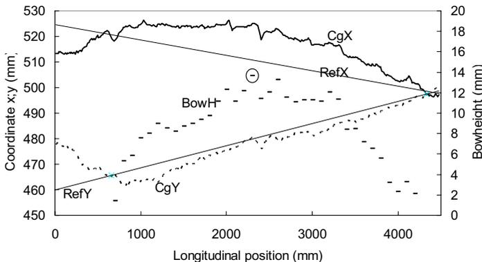
**Fig. 8.** Search for maximum (denoted by a circle) bow height (BowH). Bow height is calculated as the Euclidian distance of Center of gravity ( $C_gX$  and  $C_gY$ ) to the reference line (RefX and RefY). Example with log 1,1,1 from SPSB.
