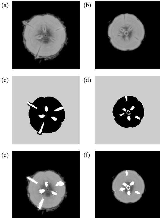
**Fig. 4.** Examples of two discs classified by an ANN with a  $7 \times 7$  input window, 15 nodes in hidden layer and one output. Original images (a) and (b), manually classified images (c) and (d), images classified by the ANN (e) and (f).
