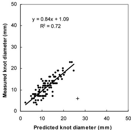
Fig. 10. Tangential knot diameter on the outer boards. Measured on real boards versus predicted by simulated sawing of corresponding boards based on parametric descriptions. Outlier (+) was excluded when fitting the regression line.
