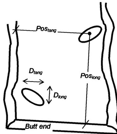
Fig. 6. Definition of measurements carried out on the real boards.
