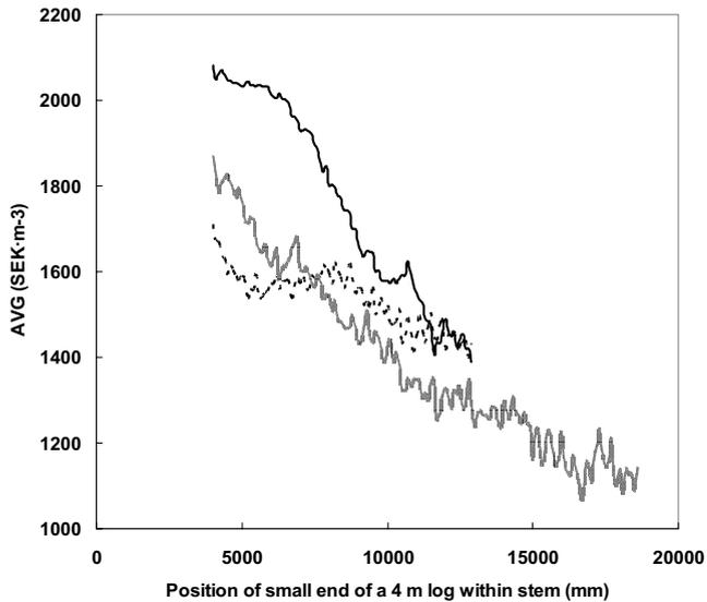
**Fig. 9.** Average board value (AVG) predicted with model M:3D on a 4-m log at different positions within stem. Example with three stems.
