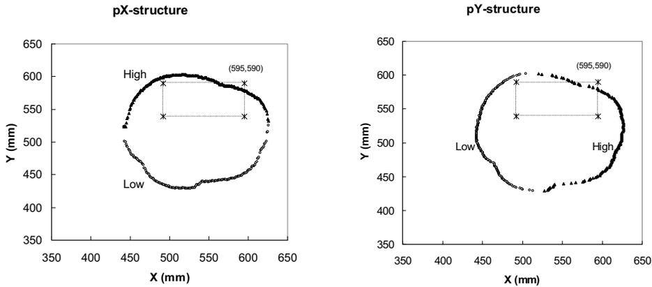
**Fig. 13.** Representation of cross-section by structures  $pX$  (left) and  $pY$  (right) after rotation and conversion. Referencing  $pX$  by an  $x$ -position the lower (low) and upper (high) extension of log is given in  $y$ -coordinates.  $pY$  works in analogy, referencing by  $y$ -positions gives extension of log in  $x$ . Example with cross-section no. 62 of log 1,1,1 from SPSB. The position of a 50x100 centre board is also shown.
