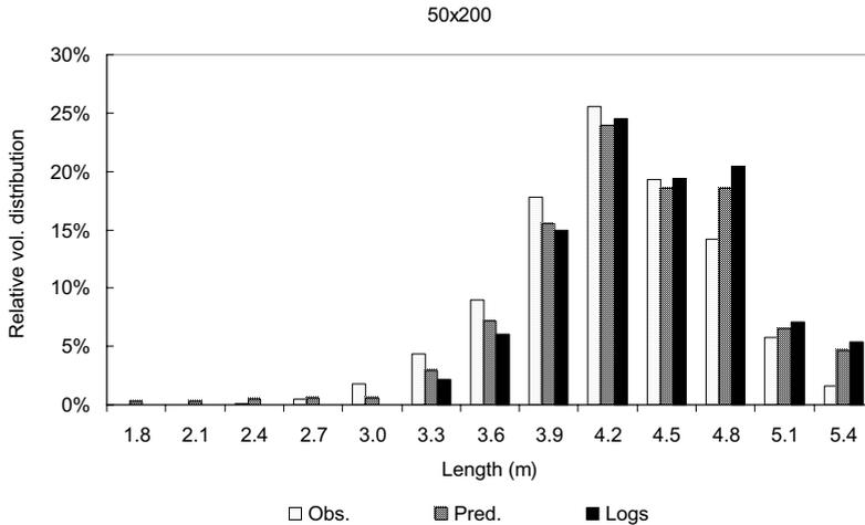
**Figure 5.** Sawmill's distribution of logs by length classes within diameters 248 mm to 261 mm SED and predicted and observed length distribution of 50- x 200-mm boards yielded from sawing the same logs. Actual log lengths within a length class were 100 mm to 399 mm longer, while logs used for simulation were 100 mm longer than length class shown.
