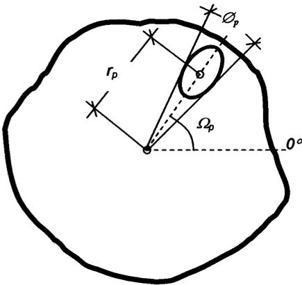
Fig. 4. Knot geometry notation, projection to a cross-section.
