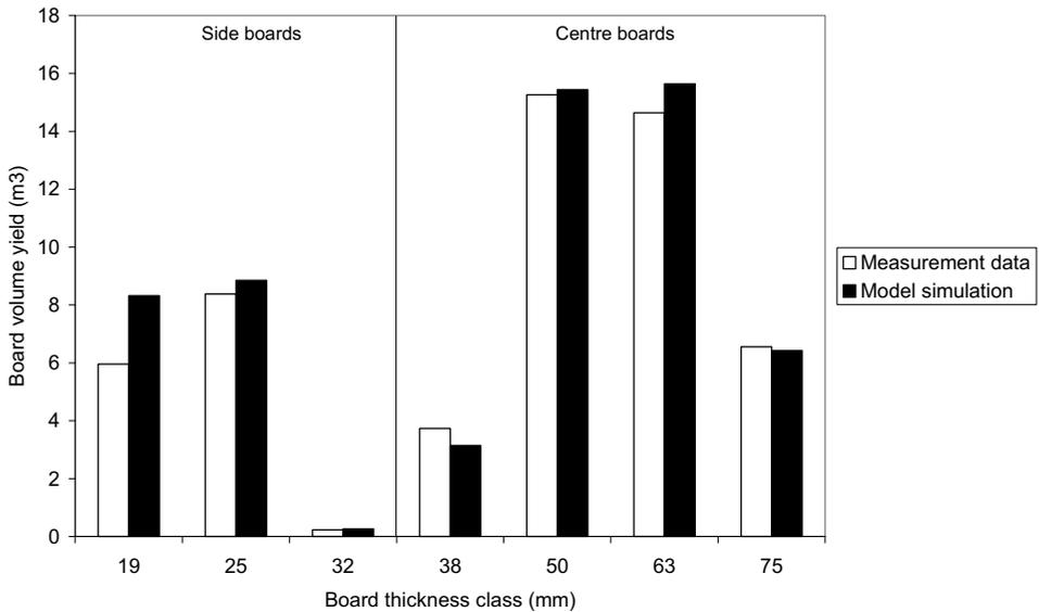
**Figure 7.** Lumber volume yield by board thickness class using tree model and empirical measurement data respectively.
