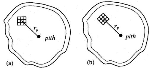
Fig. 3. Illustration of the two methods of aligning the window around the targeted pixel. (a) Horizontally aligned window, and (b) tangential alignment to the radii ( $r_p$ ) from the pith to the centre of the window.
