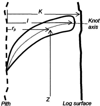
Fig. 5. Knot geometry notation, projection to a radial section.
