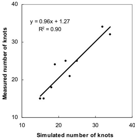
**Fig. 5.** Number of knots measured on real boards as a function of predicted number of knots based on simulated sawing of the same logs.
