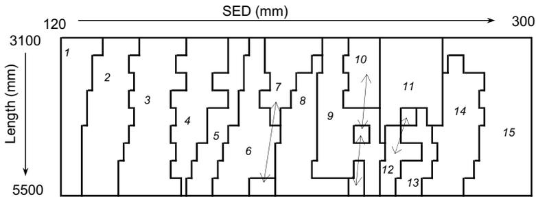
**Figure 6.** Log sorting schema obtained from value optimization with sawmill's current log distribution and with constraints on volume produced in each dimension (thickness  $\times$  width). Numbers correspond to sawing classes as in Table 1.
