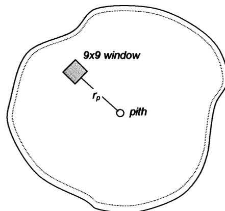
Fig. 1. Illustration of positioning of the window with the targeted pixel in the centre. As the targeted pixel scans over the computed tomographic image, interpolated greyscale values of the  $9 \times 9$  pixels in the window and the distance to pith ( $r_p$ ) are fed to the artificial neural network, which classifies the targeted pixel.
