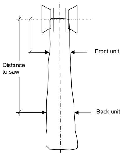
**Fig. 10.** Geometry of log centring setup. Log is individually centered at first saw and second saw respectively.
