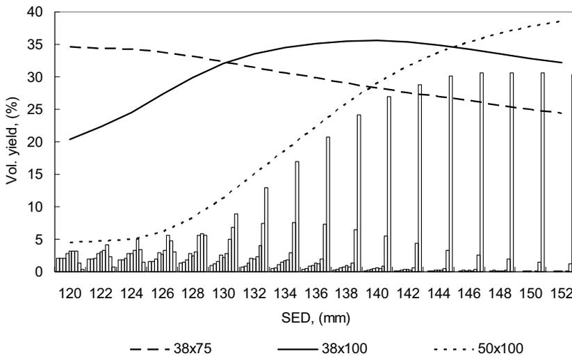
**Fig. 13.** Predicted volume yield length distribution of 38- x 100-mm boards yielded from 4300-mm-long logs with varying small-end diameter. Yield is expressed as proportion of log volume. In each presented 2-mm-wide log class, the leftmost bar represents boards 1800 mm long, and succeeding bars show boards with a 300-mm length increment up to the rightmost bar representing 4200-mm-long boards. Lines show total volume yield for three competing dimensions.
