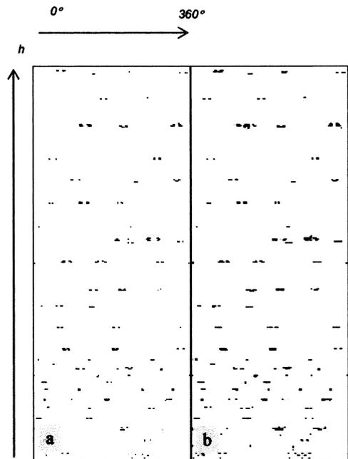
Fig. 3. Images of a concentric surface around the pith showing knots as classified by the artificial neural network (a) and after filtering (b).
