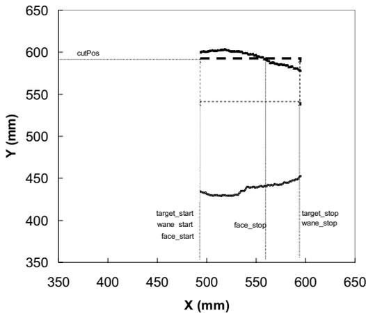
**Fig. 15.** Cutting line at  $y = 590$  on cant at cross-section no. 62, log 1,1,1 from the SPSB. The *SideProfile* of the outlined board's outside is shown. *Normal*  $(x,y,z)$  of board side is  $(0,1,0)$ .
