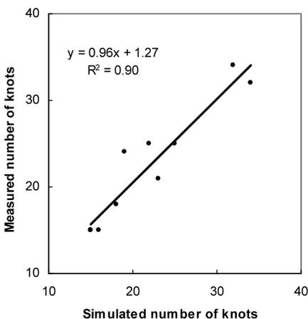
Fig. 8. Number of knots measured on the real boards as a function of simulated number of knots.
