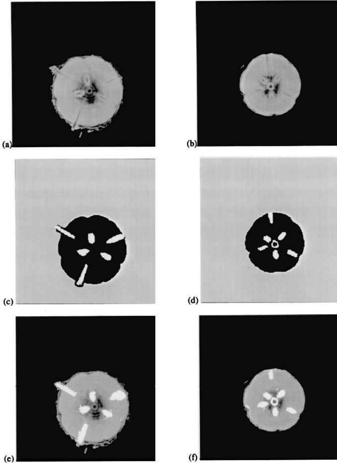
Fig. 5. Images of disc 6 (a, c, e) and disc 12 (b, d, f) classified by an artificial neural network (ANN) with the topology 50:15:1. (a, b) Original images; (c, d) manually classified images; (e, f) images classified by the ANN.
