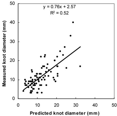
Fig. 9. Tangential knot diameter on the inner boards. Measured on real boards versus predicted by simulated sawing of corresponding boards based on parametric descriptions.
