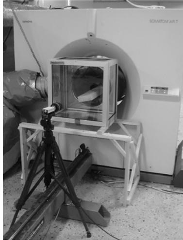
**Figure 4.** Part of the experimental setup: a digital camera and an X-ray CT scanner.
