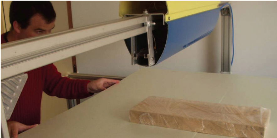
Fig. 4. Each piece of wood was placed on Styrofoam and manually fed through the scanner.
