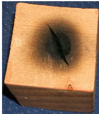
Figure 21. An internal char spot in birch wood caused by thermal runaway.
