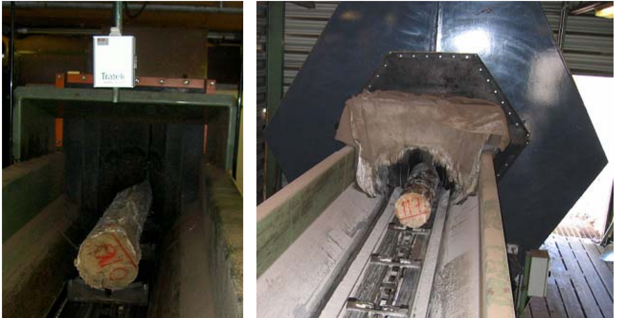
Figure 8. Scanning in X-ray (left picture) behind lead curtains. The laser spot on the surface of the log is due to the grain angle measurement, mounted above the log. 3D measurement (right picture).
