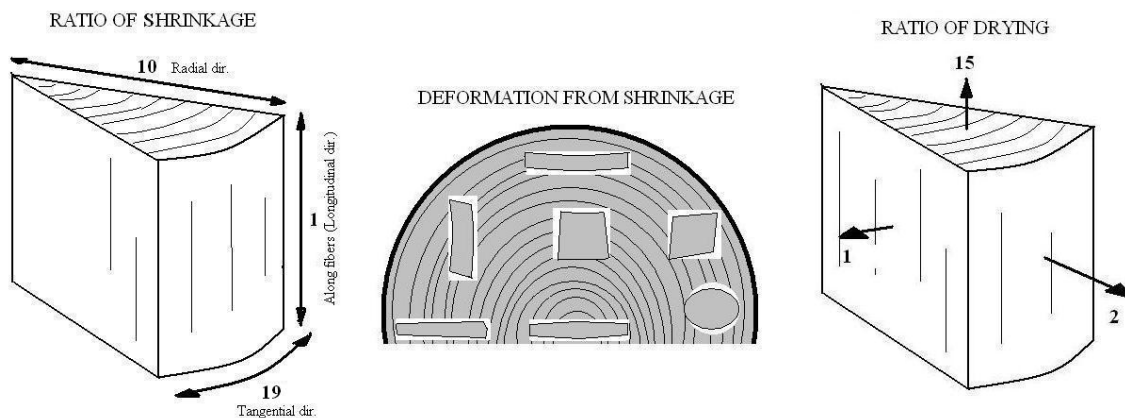
Figure 5.6, Ratio of shrinkage is different and will deform sawn timber due to location in log.
