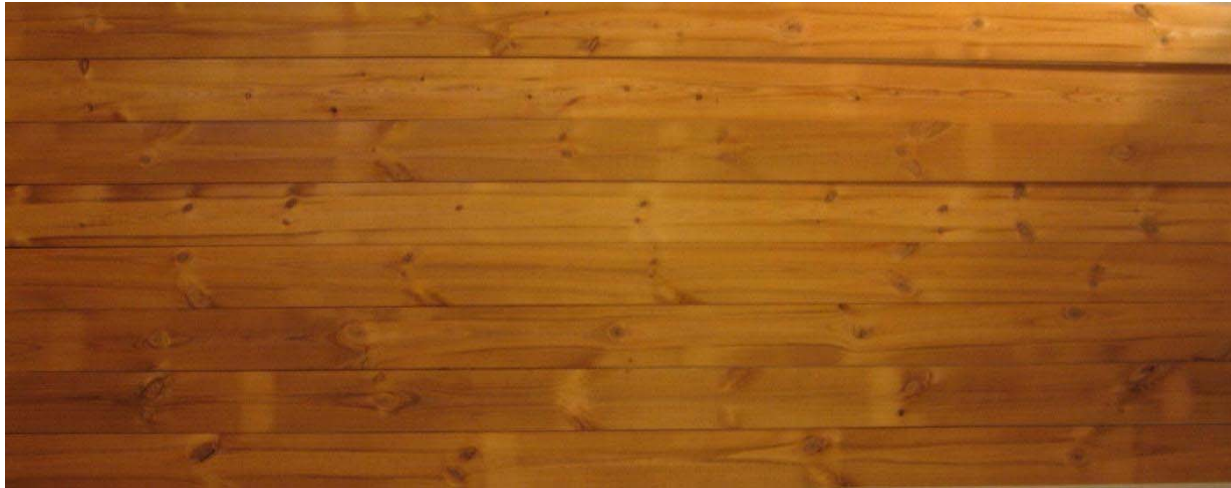
Figure 10: Sticker Staining on Planed Heat Treated Wood
