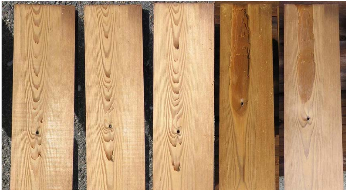
Figure 30: Multiple planing of one board sample
