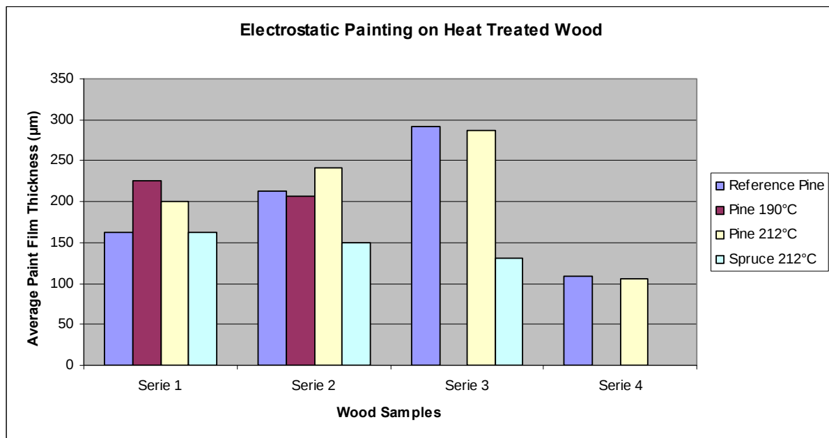
Figure 36: Paint Film Thickness from Electrostatic Painting
