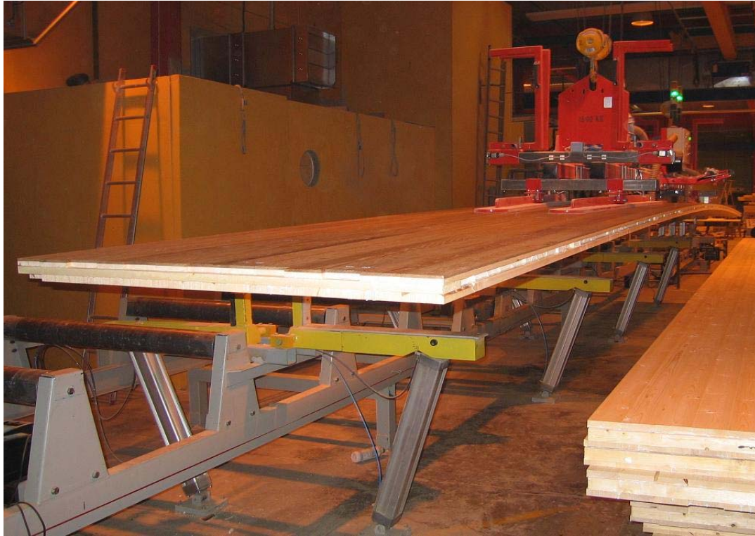
Figure 15: Oak Pine Sandwich Sheet in 12m length
