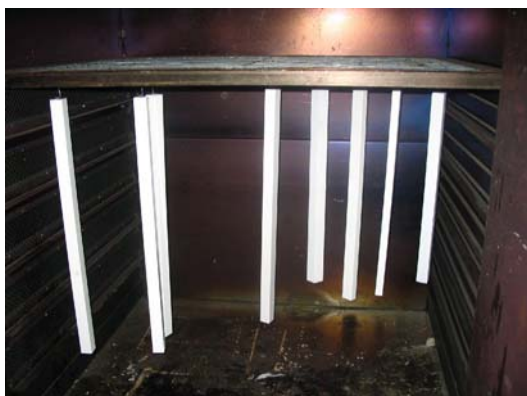
Figure 37: Oven Drying of Painted Samples
