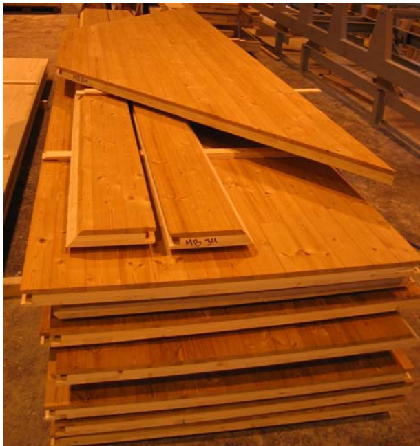
Figure 18: Massive Wood Sheets before Assembling
