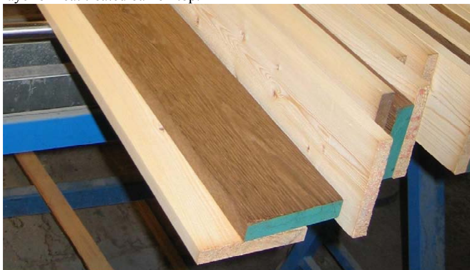
Figure 11: Oak Pine Sandwich Board Material
