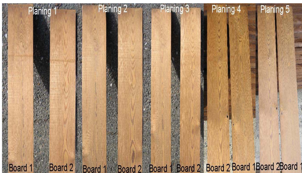
Figure 29: Planing on three sided knot free material
