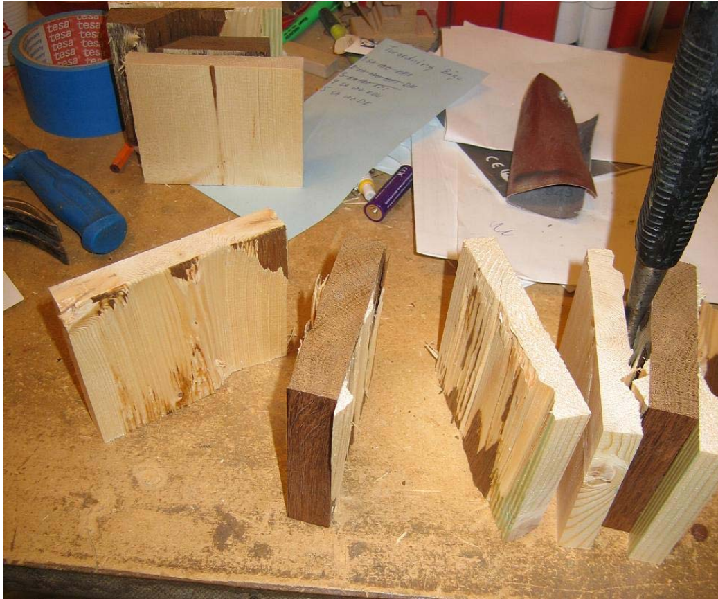
Figure 13: Glue Joint Splitting
