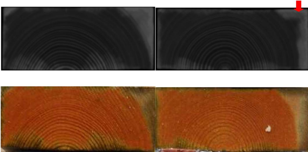
**Figure 3.30** CT-scanning image (upper) and photos taken on matched position (down) of group 2. To the left were the reconditioning samples (final MC was 17.6%) and to the right were samples dried directly to 17.6% MC after application of heartwood reagent.
