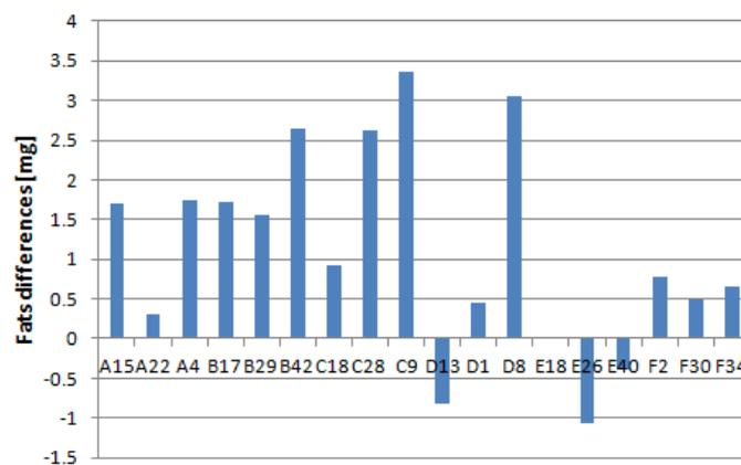
Figure 3.25 Fats difference between areas with and without impregnation failures on dried samples (the value is the amount of fats in position 4 minus that in position 5, extracted from 0.125g dry wood).
