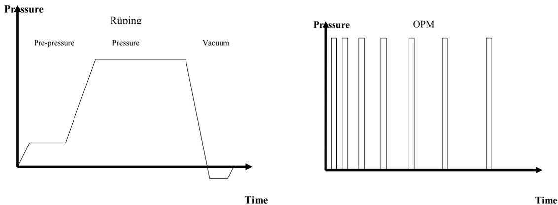
Figure 1.2 Rüping impregnation (left) and OPM impregnation (right)
