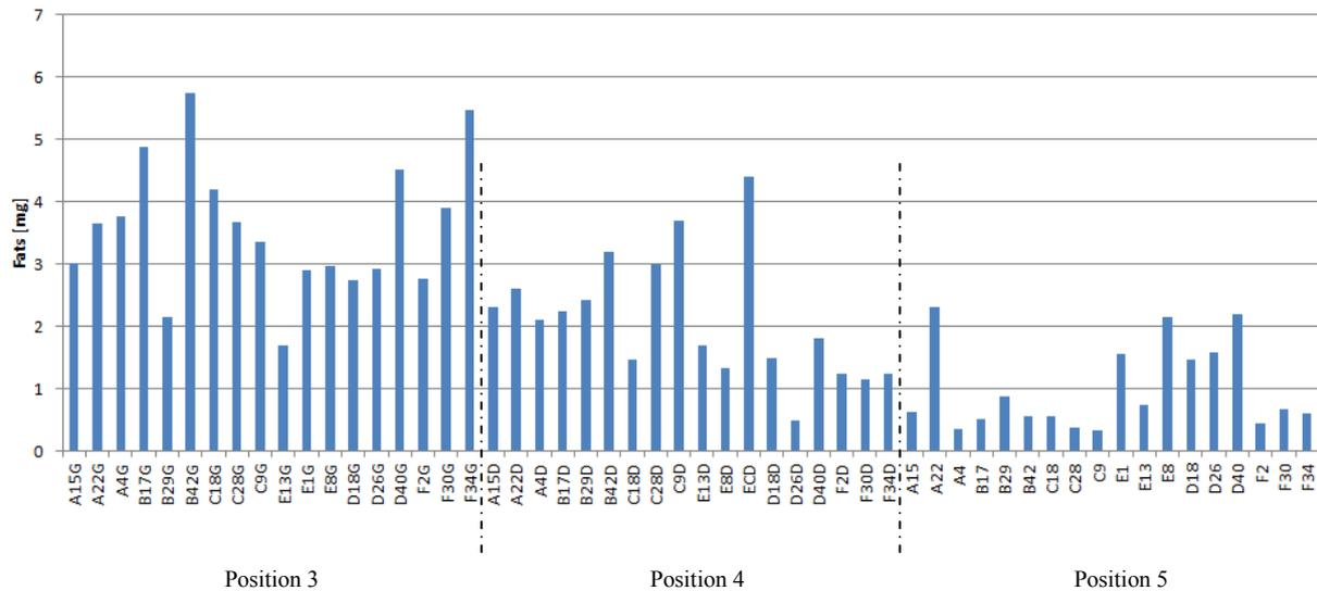
**Figure 3.18 Quantitative analysis of fats for each sample (extracted from 0.125g dry wood). Position 3: from green samples areas with failures; Position 4: from dried samples areas with failure; Position 5: from dried samples areas without failure, details see material and method.**
