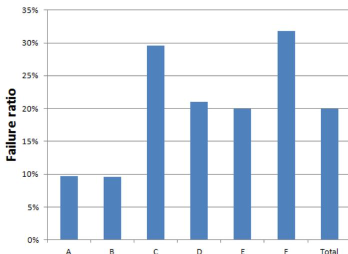
**Figure 3.2 Failure ratios of cutting surfaces at different drying temperatures and average MC: A (80°C, 20.2%), B (80°C, 13.8%), C (80°C, 8.4%), D (60°C, 22.8%), E (60°C, 16.3%), F (60°C, 8.7%).**
