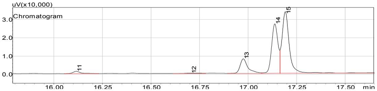
**Figure 3.16** Magnifying chromatogram of samples after transesterification from GC-FID. Peak 13 (ret. time was 16.976 min), 14 (ret. time was 17.138 min) and 15 (ret. time was 17.192 min) were fats.
