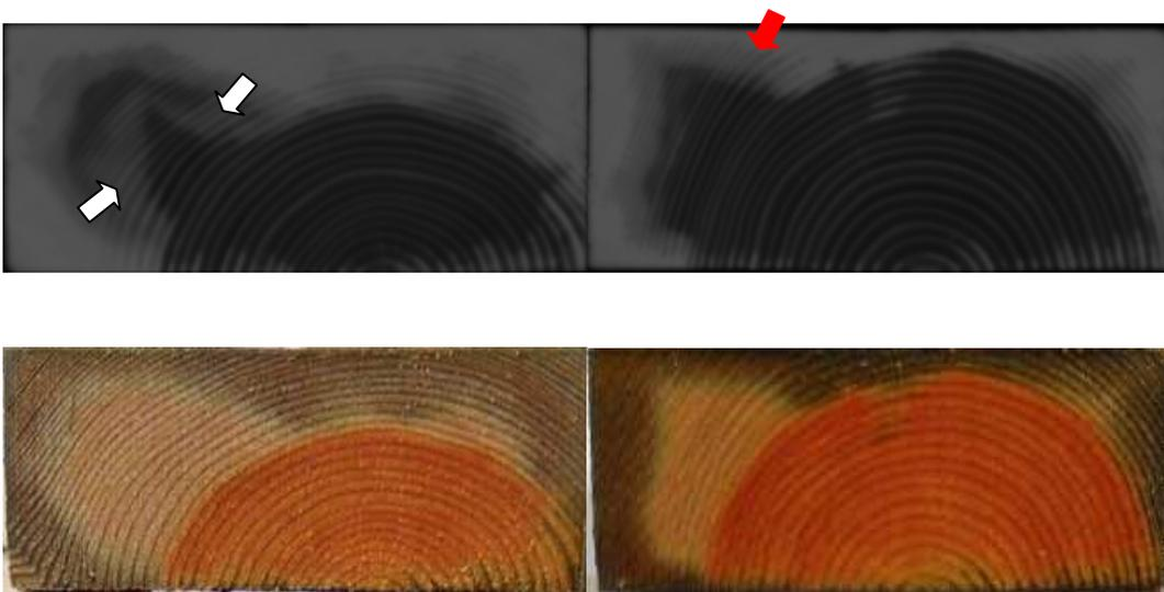
**Figure 3.31** CT-scanning image (upper) and photos taken on matched position (down) of group 3. To the left were the reconditioning samples (final MC was 17.6%) and to the right were samples dried directly to 17.6% MC after application of heartwood reagent.
