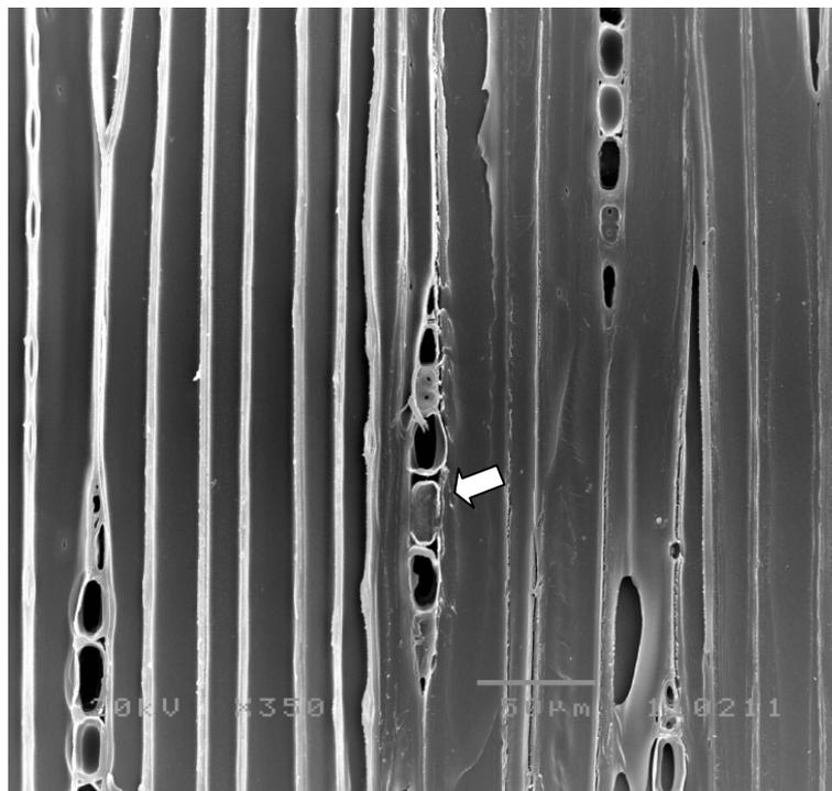
Figure 3.10 The SEM micrographs of areas with impregnation failures (tangential-section). The parenchyma cell was filled with resin (arrowhead).
