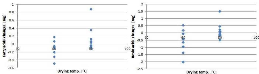
**Figure 3.22 Fatty acids (left) and resin acids (right) changes (the amount of fatty acids and resin acids in position 4 – those in position 3) VS drying temperature in extracts from 0.125g dry wood.**
