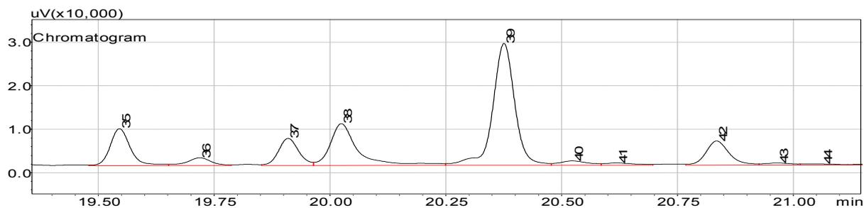
**Figure 3.13** Magnifying chromatogram of samples after trimethylsilylation from GC-FID. Peak 38 (ret. time was 20.024 min) was fatty acids, peak 39 (ret. time was 20.375 min) and 42 (ret. time was 20.834 min) were resin acids.
