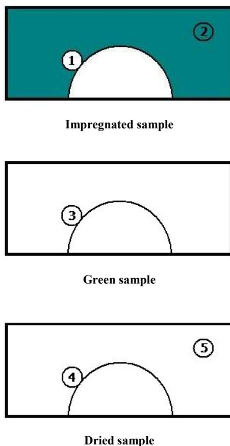
**Figure 2.3** Locations from which sawdust for extraction and GC-analysis was isolated (1 and 2 are reference points, 3, 4 and 5 were locations from which sawdust were made)
