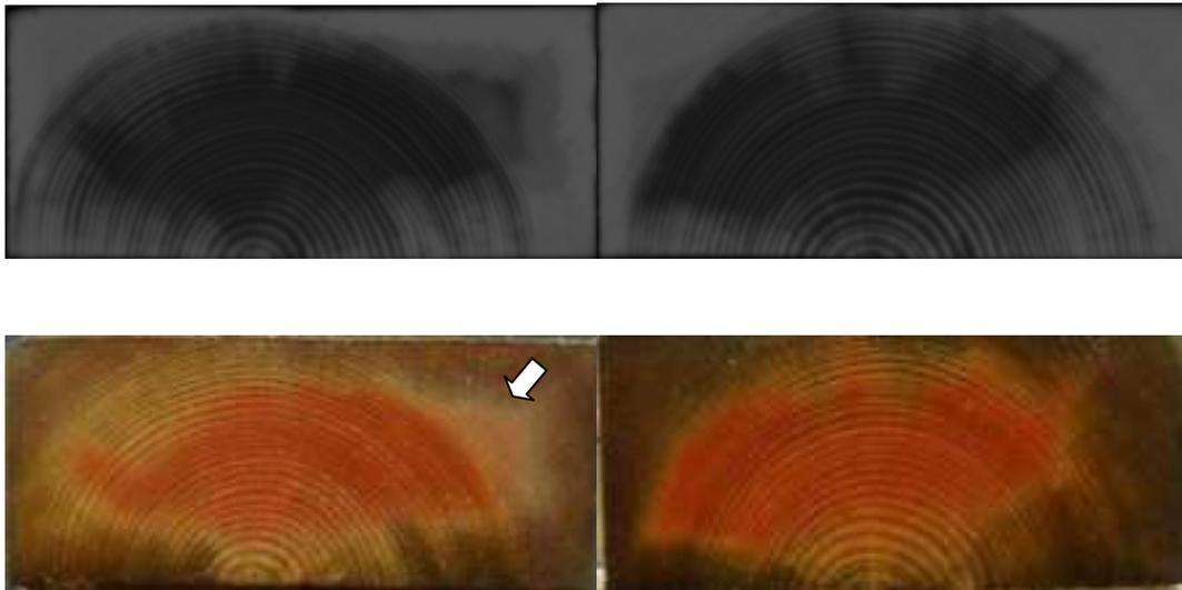
**Figure 3.32 CT-scanning image (upper) and photos taken on matched position (down) of group 4. To the left were the reconditioning samples (final MC was 17.6%) and to the right were samples dried directly to 17.6% MC after application of heartwood reagent.**
