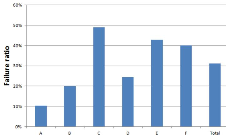
Figure 3.1 Failure ratios of boards at different drying temperatures and average MC: A (80°C, 20.2%), B (80°C, 13.8%), C (80°C, 8.4%), D (60°C, 22.8%), E (60°C, 16.3%), F (60°C, 8.7%).
