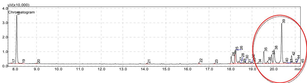
Figure 3.12 Chromatogram of green samples after trimethylsilylation from GC-FID. Peak 18 was naphthalene, peak 38 was fatty acids, peak 39 and 42 were resin acids.
