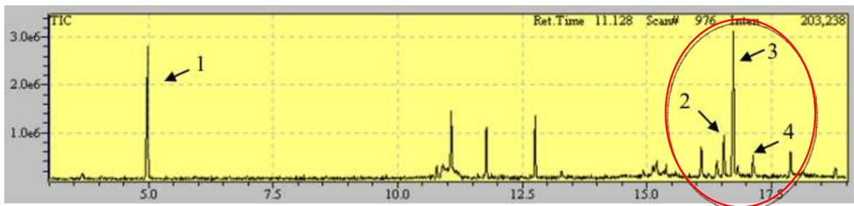
Figure 3.11 Chromatogram of green samples after trimethylsilylation from GC-MS. Peak 1 was naphthalene, peak 2 was fatty acids, peak 3 and 4 were resin acids.
