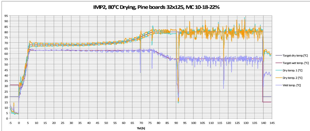
Figure 2.2 Drying scheme at 80°C
