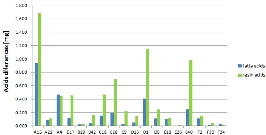
Figure 3.24 Fatty acids and resin acids difference between areas with and without impregnation failures on dried samples (the value is the amount of fatty acids and resin acids in position 4 minus those in position 5, extracted from 0.125g dry wood).
