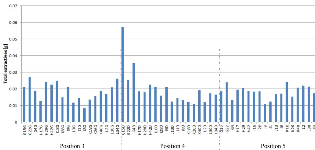
**Figure 3.26** Total extractives in 0.5g dry wood. Position 3: from green samples areas with failures; Position 4: from dried samples areas with failure; Position 5: from dried samples areas without failure, details see material and method.
