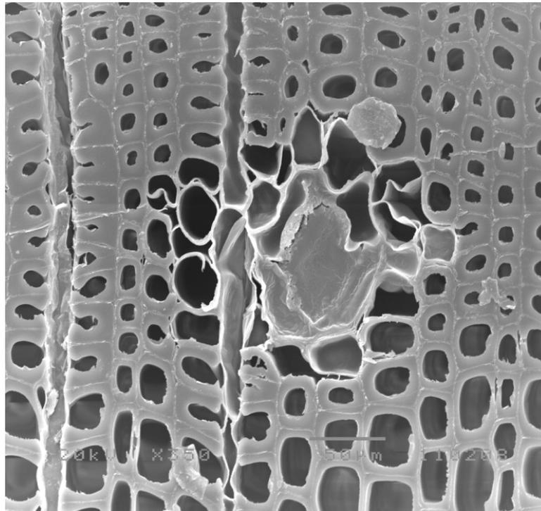
Figure 3.9 The SEM micrographs of areas with impregnation failures (cross-section). The resin canal was filled with resin.
