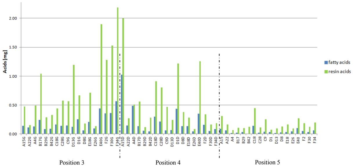
**Figure 3.17** Quantitative analysis of fatty acid and resin acid for each sample (extracted from 0.125g dry wood). Position 3: from green samples areas with failures; Position 4: from dried samples areas with failure; Position 5: from dried samples areas without failure, details see material and method.
