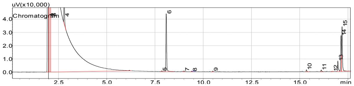
**Figure 3.15** Chromatogram of samples after transesterification from GC-FID. Peak 6 was naphthalene, peak 13, 14 and 15 were fats.
