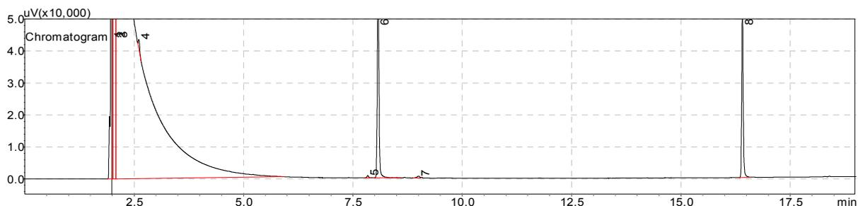
**Figure 3.14** Chromatogram of pure fats after transesterification from GC-FID. Peak 6 was naphthalene, peak 8 was pure fats.
