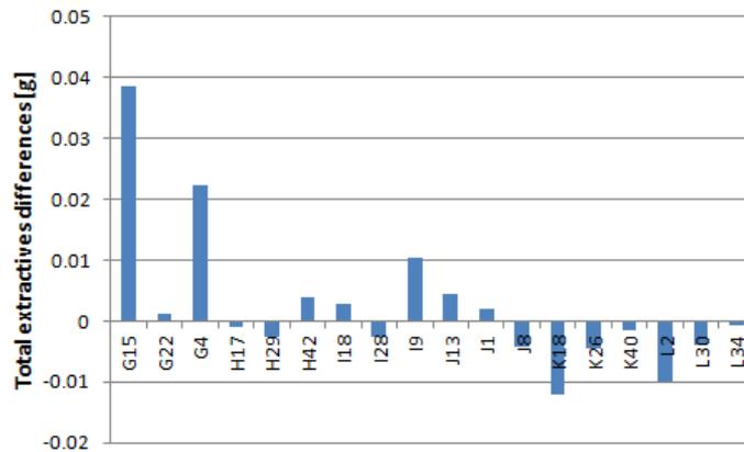
Figure 3.28 Total extractives differences (in 0.5g dry wood) between areas with and without impregnation failures on dried samples (the amount of total extractives in position 4 minus those in position 5).
