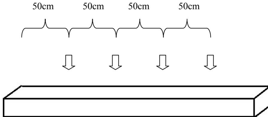
**Figure 2.3 Cutting positions after impregnation**
