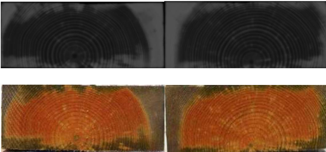
**Figure 3.29** CT-scanning image (upper) and photos taken on matched position (down) of group 1. To the left were the reconditioning samples (final MC was 17.6%) and to the right were samples dried directly to 17.6% MC after application of heartwood reagent.
