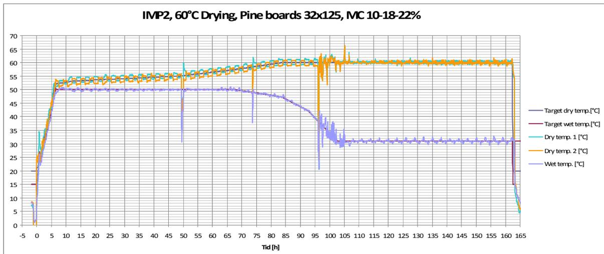
Figure 2.1 Drying scheme at 60°C
