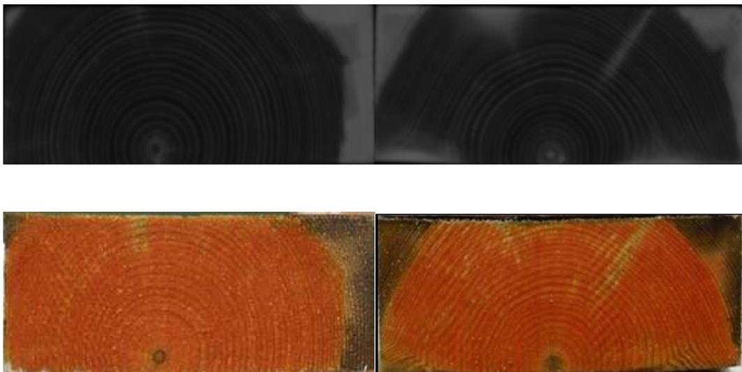
**Figure 3.33 CT-scanning image (upper) and photos taken on matched position (down) of group 5. To the left were the reconditioning samples (final MC was 17.6%) and to the right were samples dried directly to 17.6% MC after application of heartwood reagent.**
