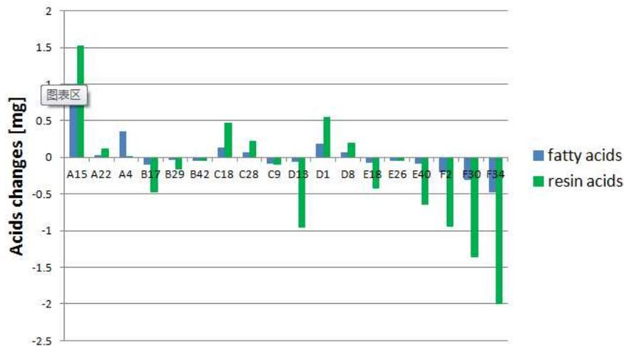
Figure 3.19 Fatty acids and resin acids changes between green and dried samples (the amount of acids in position 4 minus those in position 3), extracted from 0.125g dry wood.
