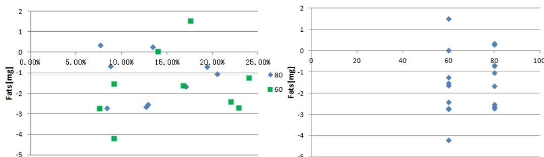
**Figure 3.23 Fats changes (the amount of fats in position 4 – those in position 3) VS moisture content as well as drying temperature in extracts from 0.125g dry wood.**
