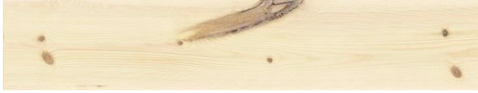
Figure 2.5: Board with a very steep splay knot. Most likely due to a top rupture.
