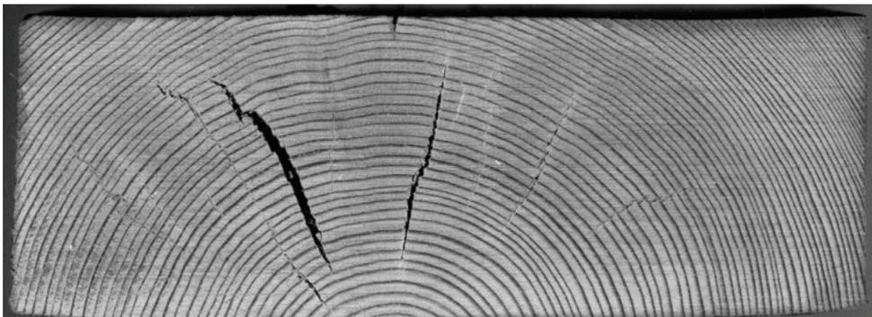
*Figure 1: Example of internal checking of heat treated spruce.*
