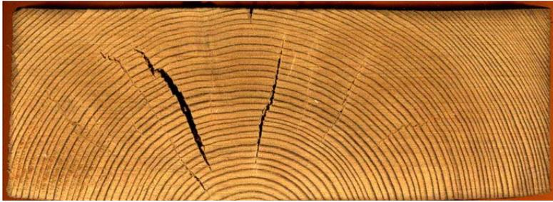
**Figure 1.** Internal checking in spruce caused by heat treatment.
