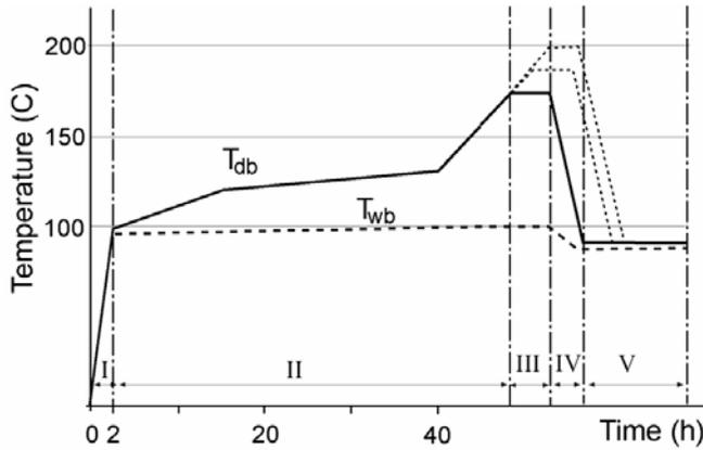
**Figure 2:** Treatment process divided into five regimes. I) Heating with superheated steam. II) Drying regime – High temperature drying: the wood reaches almost 0% MC. III) Treatment regime –Wet bulb temperature kept at 99°C by continuously injecting steam as shielding gas. IV) Cooling regime – Cooling rate is regulated with the electric heating coil, steam and water spray. V) Conditioning regime – The objective of this regime is cooling and remoistening.
