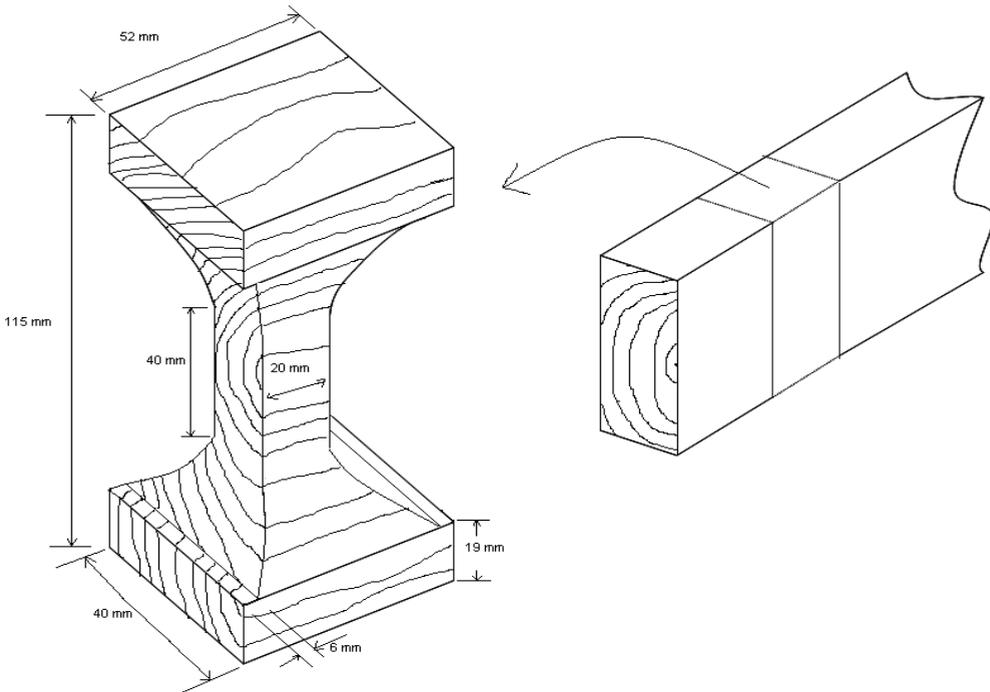
**Figure 16:** Samples for tensional strength test in tangential direction. This design was used both for comparison of the two different reference groups in paper III and in a small study of the effect of high temperatures on tensional strength.
