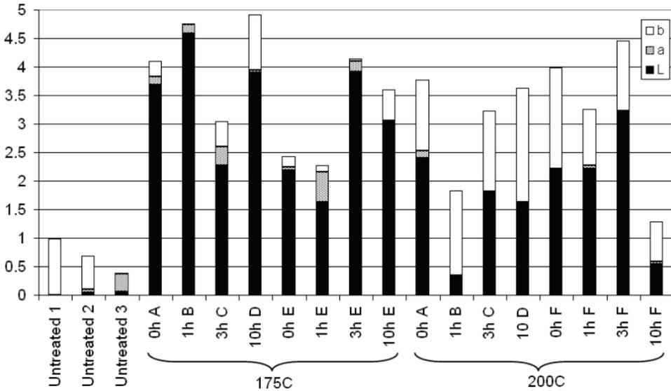
**Figure 8:** Colour heterogeneity values of birch boards subjected to different heat-treatment processes. Each bar shows the heterogeneity of one board. The different colours in each bar represent the different colour coordinates' contribution to the heterogeneity. (Figure from paper I)
