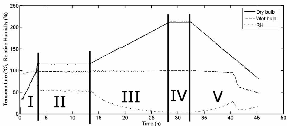
**Figure 3.** Heat treatment schedule used in this work. The process can be divided into five regimes: I Heating, II 1st drying, III 2nd drying, IV Treatment, V Cooling regime.
