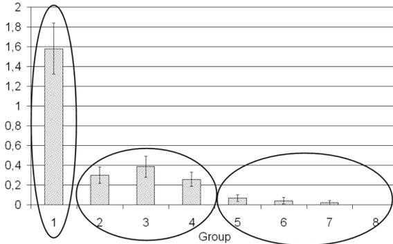
**Figure 4:** Mean number of internal checks per cross section together with bars showing the 95% confidence interval. Circles show groups with statistically significant different number of internal checks with 95% confidence.
