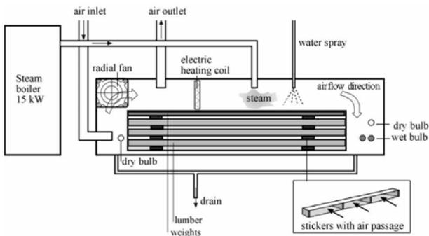
**Figure 1:** Kiln for thermal treatment of wood by using superheated steam as shielding gas.
