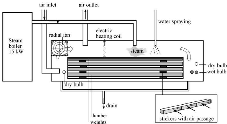
**Figure 2.** Experimental kiln for heat treatment of wood.
