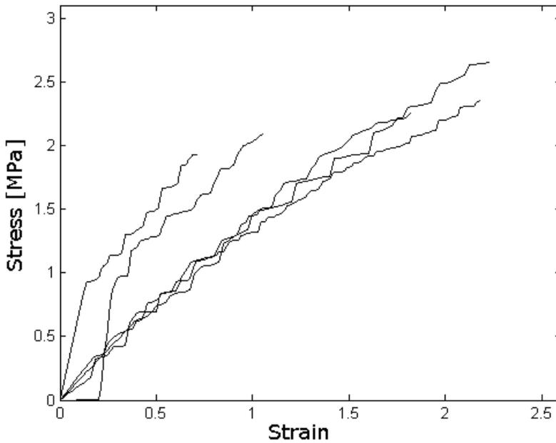
**Figure 19:** Testing of tensile strength in the tangential direction in spruce. Testing was performed in an oven heated to 180°C.
