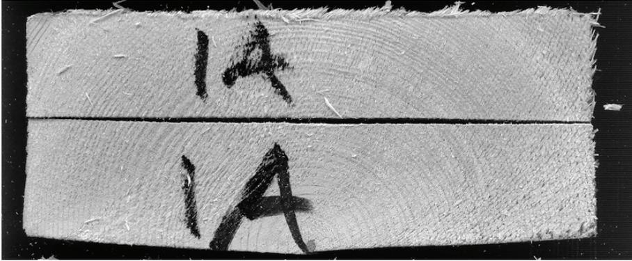
**Figure 5:** Slicing test from high temperature dried reference boards. Gap due to approximately 1 mm. Samples were cut after the 1<sup>st</sup> drying regime.
