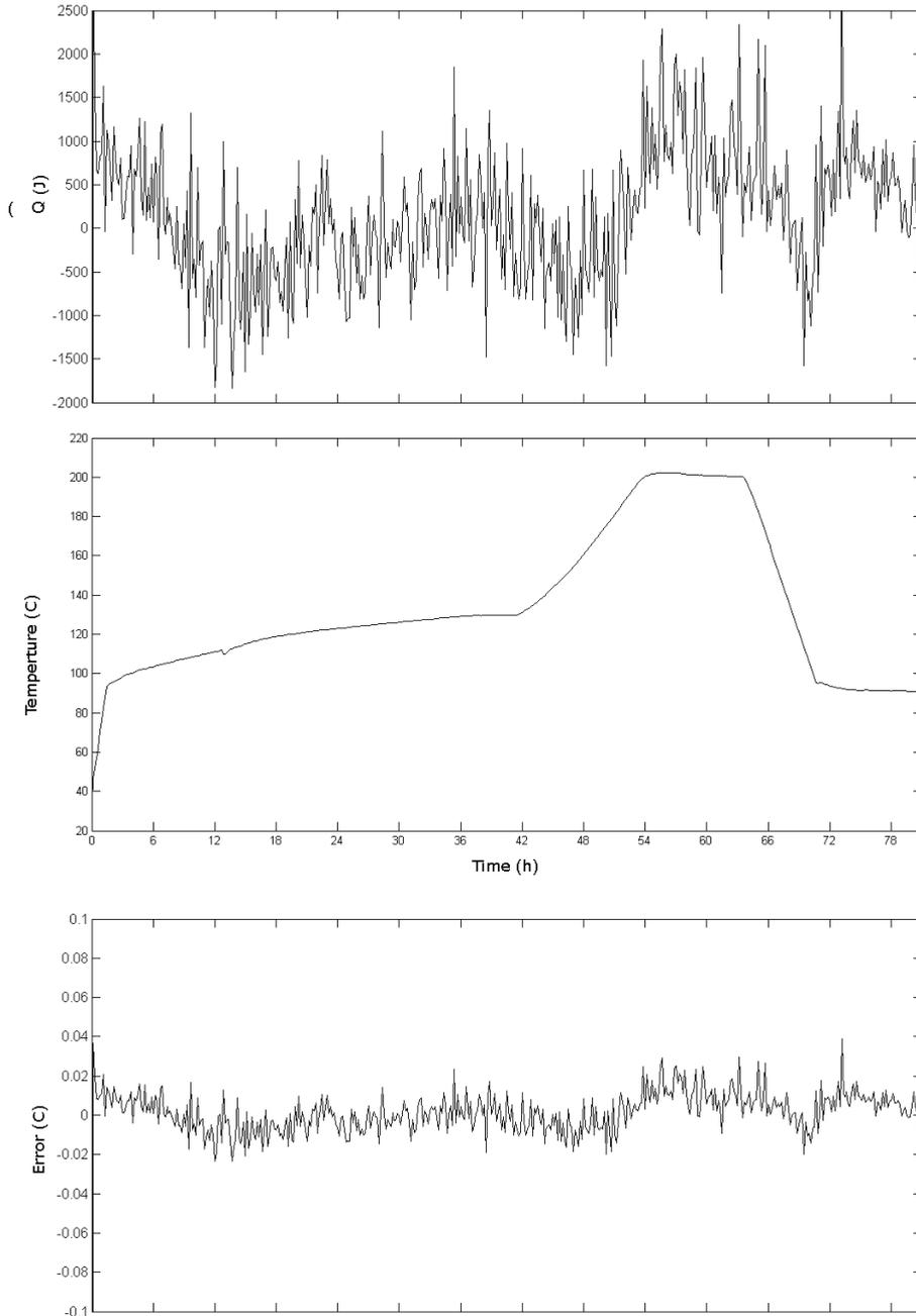
**Figure 12a-c:** a) The calculated source term  $Q$ . b) The temperature measured closest to the surface. c) Shows the error; i.e., the difference between calculated and measured internal temperature after calculating  $Q$ .
