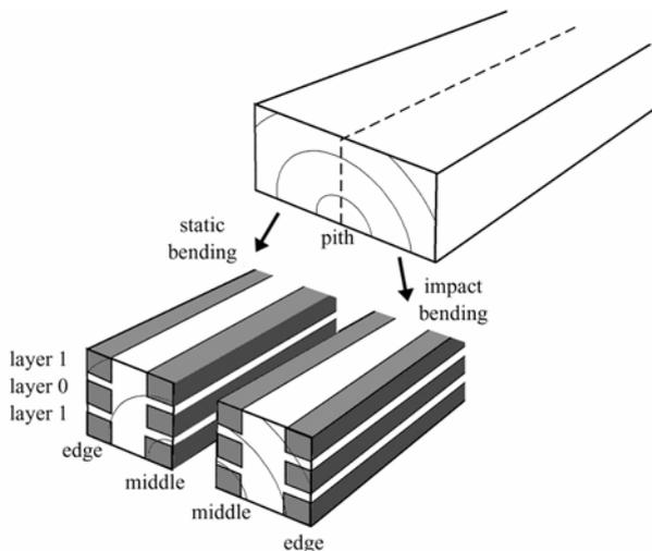
**Figure 3:** Method for selecting test samples for static- end impact bending tests.
