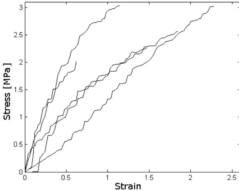
**Figure 18:** Testing of tensile strength in the tangential direction in spruce. Testing was performed in an oven heated to 150°C.
