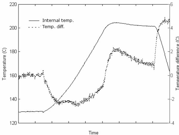
**Figure 8:** Internal temperature and its difference to the temperature at the surface of the board (internal temperature – surface temperature).
