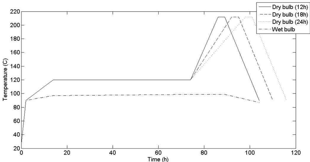
**Figure 15:** The three different process schedules used in paper III. For each process with different time span, two batches were treated, one with 18% initial MC and one with 6% initial MC. A seventh process was used as reference. Both initial MC levels were included, but the treatment was stopped at the end of the 1<sup>st</sup> drying regime.
