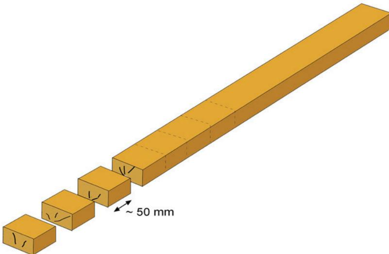
**Figure 13:** Method used for detecting internal checking. The board is cut and one cross-section surface is visually graded. For each visually graded surface, the number of internal checks, knots, checks in knots and presence of pith are documented.
