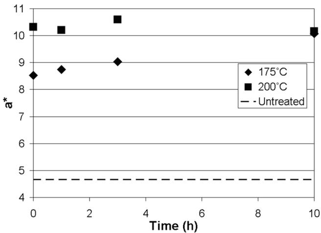
**Figure 10:** Average values in yellowness ( $a^*$ ) for all measurement done in the different heat-treatment processes. (Figure from paper I)
