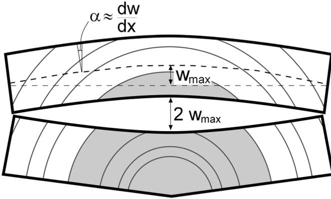
**Figure 6:** The measured gap in the slicing test is assumed to be twice the deflection of each part. It is also assumed that the centre lines of the two parts are sinus function along the dotted line.
