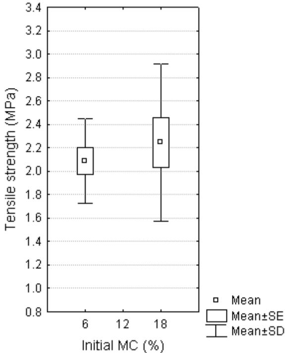
**Figure 17:** Tensile strength in the tangential direction for the two reference groups in paper III.
