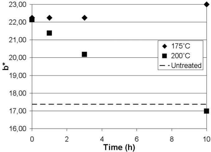
**Figure 11:** Average values in redness ( $b^*$ ) for all measurement done in the different heat-treatment processes. (Figure from paper I)
