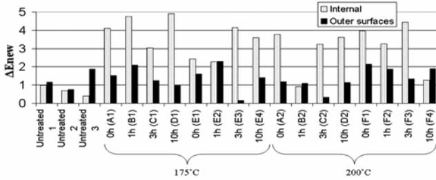
**Figure 7:** The internal colour difference  $\Delta E_{new}$  and the colour difference between the outer surfaces of the board.
