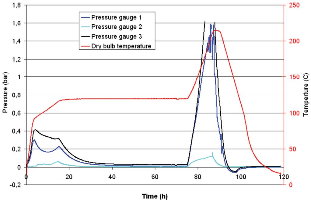
**Figure 14:** Treatment temperature plotted together with pressure. Maximum pressure is reached in the second drying regime, which suggests that the pressure is most likely due to vapour and thermal expansion. The low value of the pressure gauge may be an affect of leakage.
