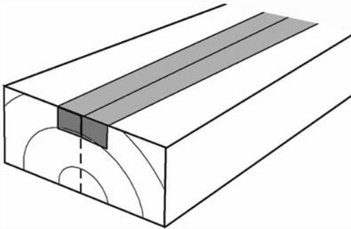
*Figure 4: Positions from which the samples for matched-pair testing were taken.*
