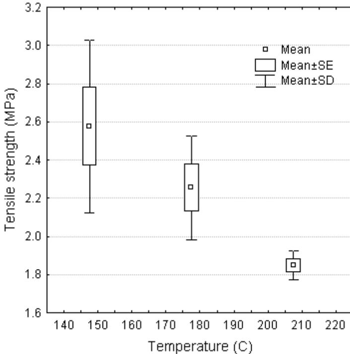
**Figure 21:** Tensile strength in the tangential direction of spruce at 150°C, 180°C and 210°C.
