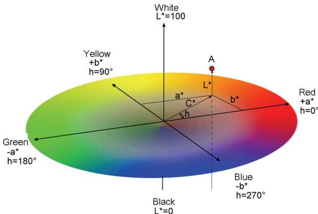
**Figure 6:** The three-dimensional CIE  $L^*a^*b^*$  colour space. The  $L^*$  coordinate is the level of lightness. The  $a^*$  and  $b^*$  coordinates give the colour of the measurement. The figure also shows how the colour can be described with the polar coordinates  $C^*$  (saturation) and  $h$  (hue angle).
