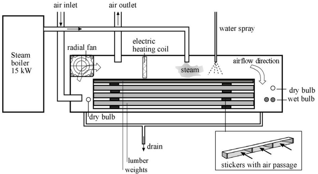
**Figure 3:** Graphical description of the kiln. All basic functions of an industrial drying kiln are present. The radial fan makes it impossible to reverse the airflow as is done industrially. Due to the limited size, stickers with air passages were designed. (Figure from papers I & II)
