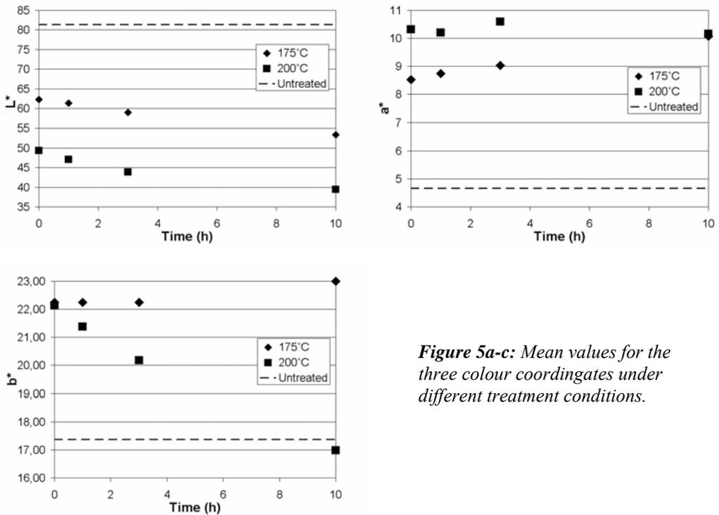
**Figure 5a-c:** Mean values for the three colour coordinates under different treatment conditions.
