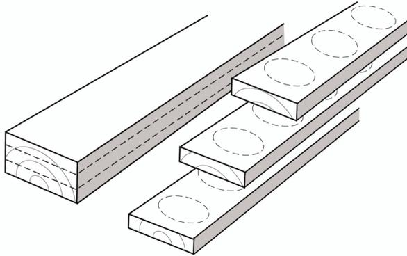
**Figure 5:** Cutting of board to measure colour through the board's thickness. Colour measurements were performed on both sides of every slice through the board.
