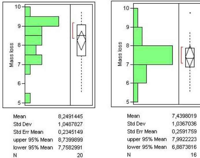
**Figure 7.** Distribution of mass loss in heat treated boards. Left side is the distribution of mass loss of boards with internal checking. Right side is the distribution of mass loss of boards without internal checking.
