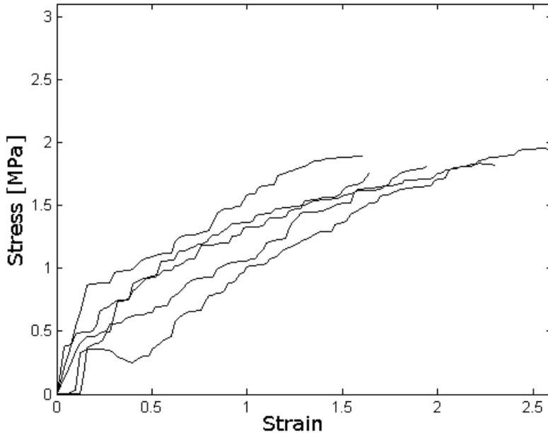
**Figure 20:** Testing of tensile strength in the tangential direction in spruce. Testing was performed in an oven heated to 210°C.
