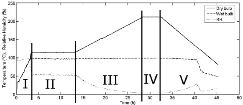
**Figure 1:** Process schedules used in the experiment. Dotted line shows relative humidity. Process is divided into five regimes. I) Heating regime II) 1<sup>st</sup> Drying regime III) 2<sup>nd</sup> drying regime IV) Treatment regime V) Cooling regime (Figure from paper II)
