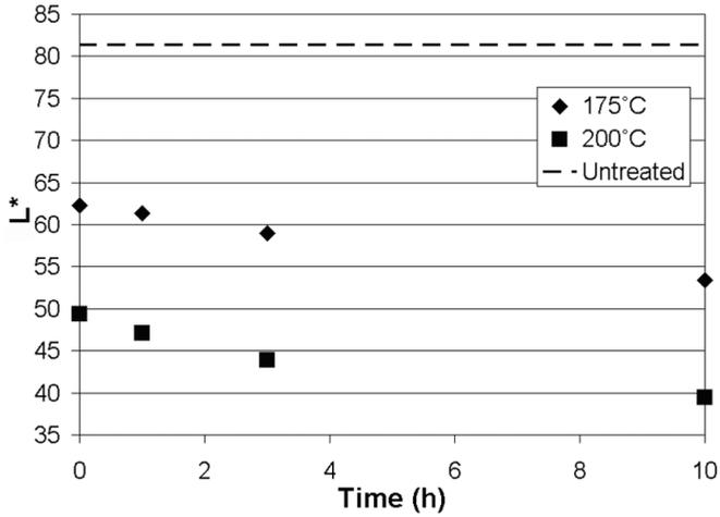
**Figure 9:** Average values in lightness ( $L^*$ ) for all measurement done in the different heat-treatment processes. (Figure from paper I)
