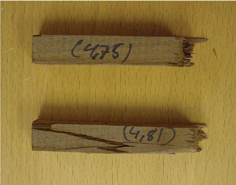
**Figure 4:** The two different types of fractures defined in the impact testing. Top: ordinary fracture; bottom: shear fracture.
