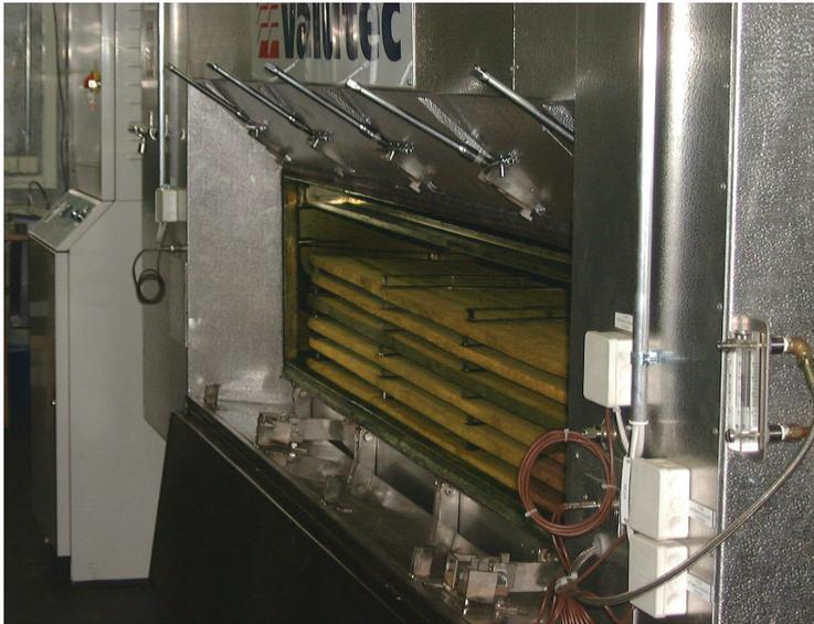
*Figure 2: The experimental kiln used for heat treatments at Luleå University of Technology. Due to the size of the kiln, the batch size is limited to less than half a cubic meter.*
