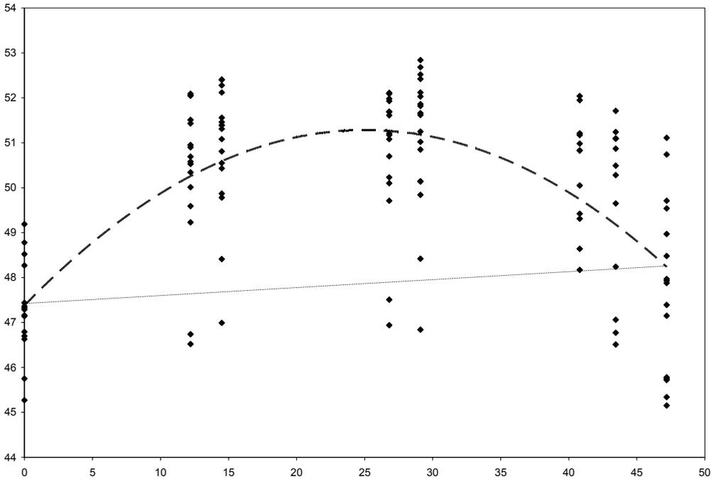
**Figure 7:** The *L* coordinate measured at eight positions through a board. The dashed line shows the second degree polynomial fitted to the measurement, and the solid line the linear part of the polynomial.
