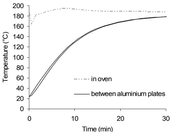
**Figure 4.** The measured temperature in the oven and between the aluminium plates as a function of time. The oven temperature was 180°C.
