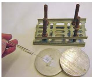
**Figure 6.** A carboxylic acid is added to the filter paper on the aluminium plate. The frame that clamps the two plates together during esterification is in the background.
