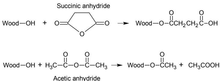
**Figure 5.** Modification reactions between wood and succinic or acetic anhydride.
