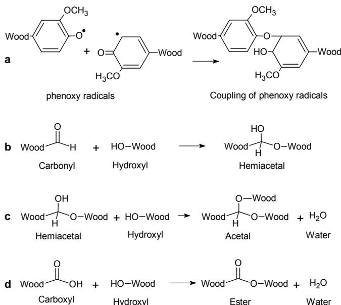
**Figure 3.** Some proposed adhesion mechanisms in the environmentally friendly boards.
