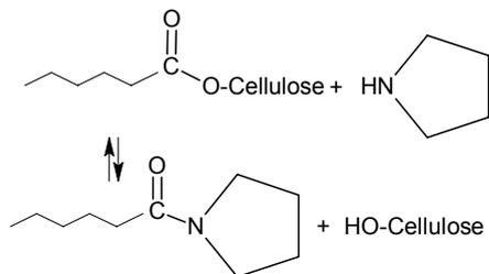
**Figure 5.** Aminolysis of cellulose hexanoate. Pyrrolidine reacts with the ester and forms hexanoyl pyrrolidine.
