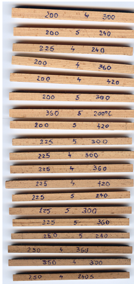
Fig. 5.2 Scanned image of 19 samples. The numbers stand for the pressing parameters used to manufacture them (plate temperature, pressure, time)
