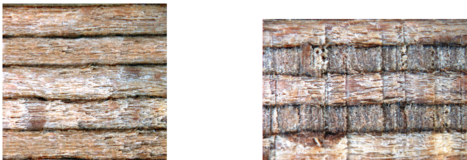
Fig 3.2. Longitudinal section of a – parallel-grained , b – cross-grained board; microscopical view (7x magnification)
