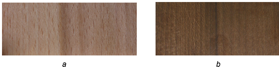
Fig. 5.1 Beech veneer with red heartwood before and after pressing.
