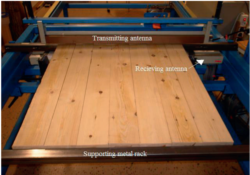
Figure 11. Satimo microwave equipment. The two antennas and one of the supporting metal racks are marked in the figure.
