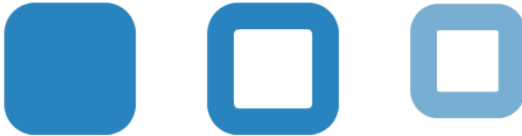
Figure 1. Schematic picture of water in a wood cell. To the left is a fully saturated cell, in which the entire lumen is filled with water. In the centre is a cell at the fibre saturation point, at which the lumen is empty but the cell wall remains fully saturated. To the right is a cell at a moisture content value below the fibre saturation point, at which the cell wall also contains less water and has started to shrink.
