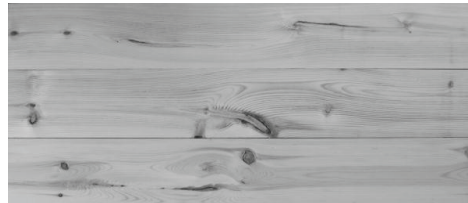
Figure 5. Three characteristic boards from the group “Defect”. Note the grain deviations in large areas.
